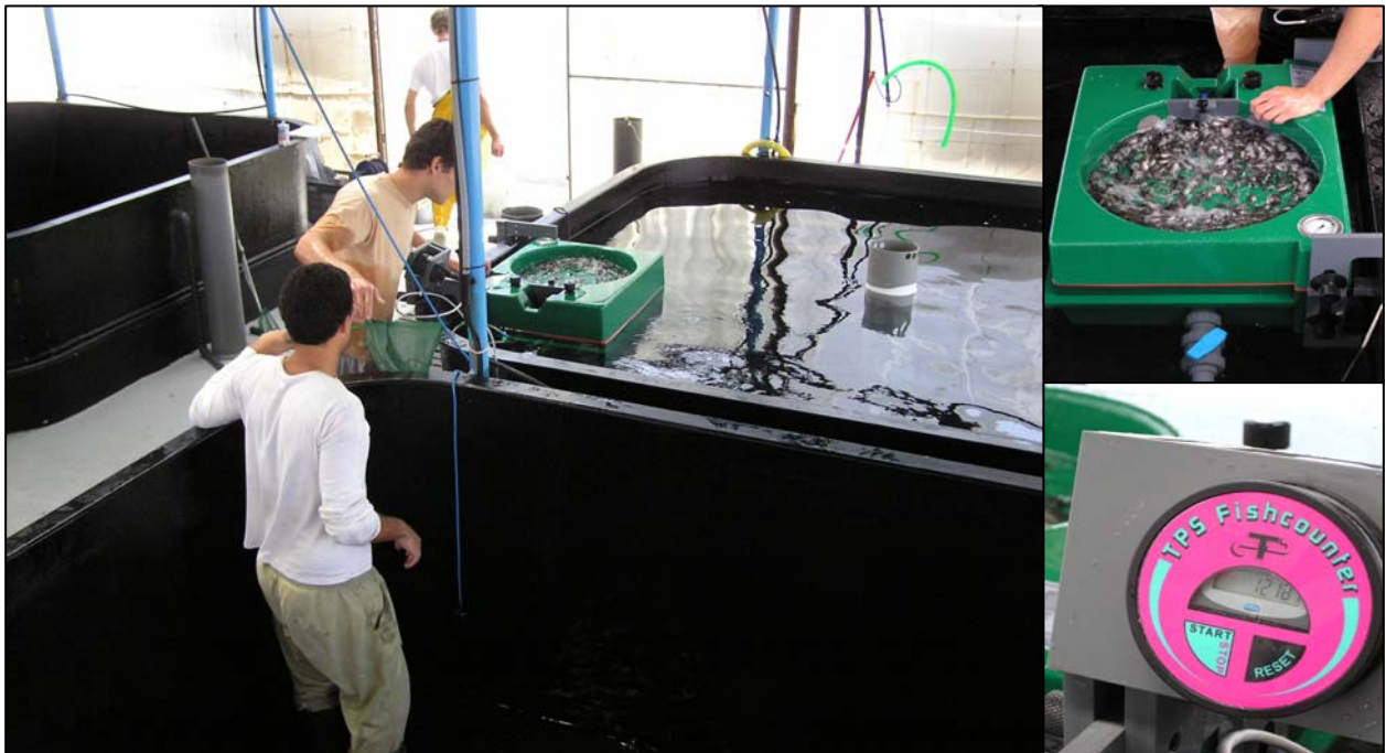
Figure 50. a) Automatic fry count; c,d) details of automatic fry counter TPS Fishcounter.
