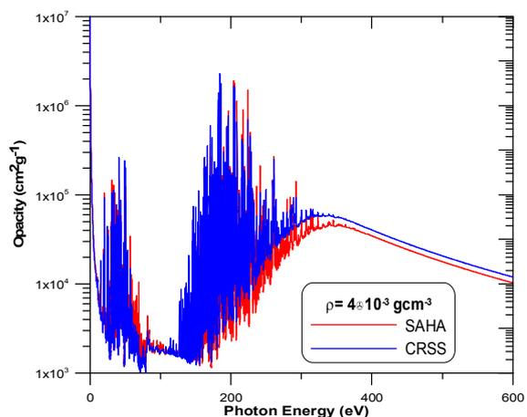
Figure 2. Spectrally resolved opacity.
