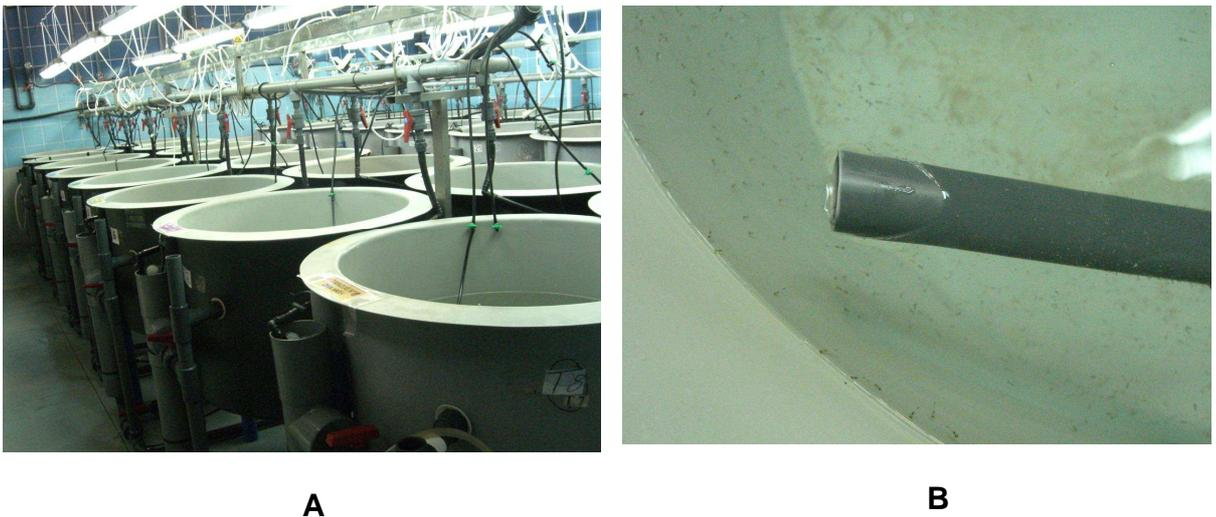
**Figure 9 A:** experimental cylindro - conical tanks used in trial II. **B:** surface skimmer used to clean the surface of the tanks.
