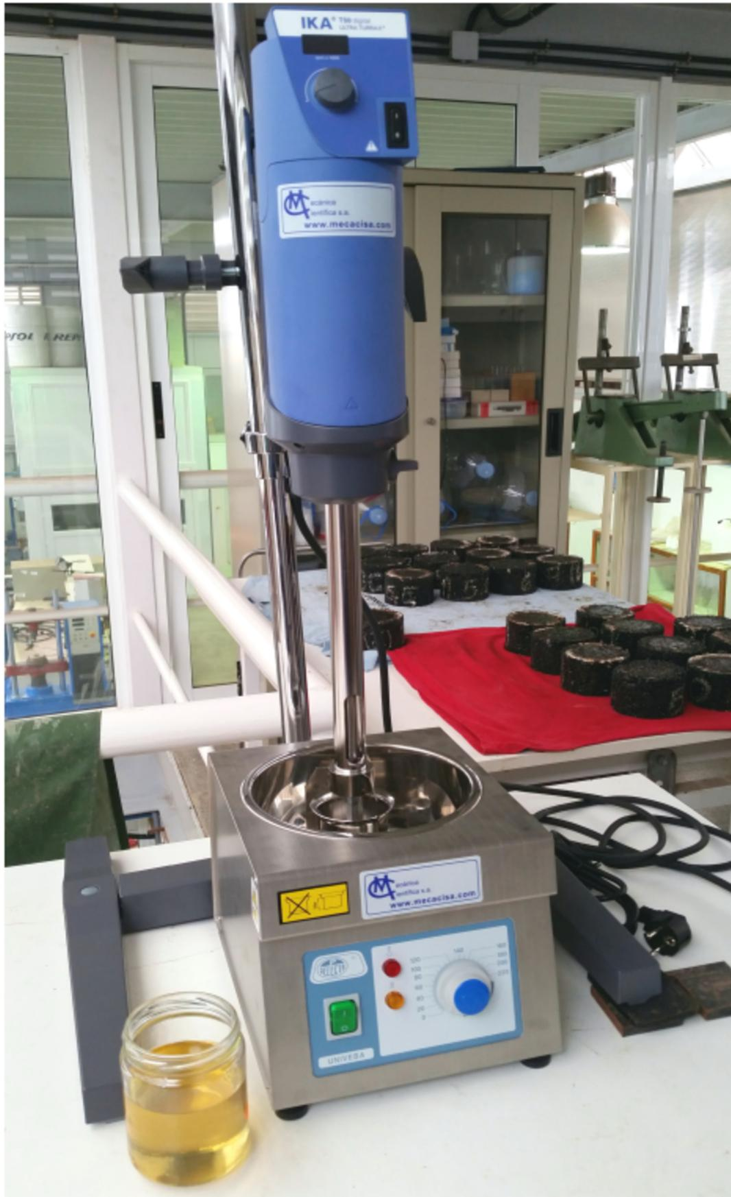
**Fig. 2.** Mixer unit employed to prepare the AR binder containing WMA additive. In the foreground, liquid WMA additive.
