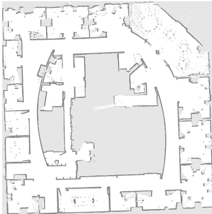
Figure 9.3: Occupancy grid map. Interior of the Intel Research Lab in Seattle
