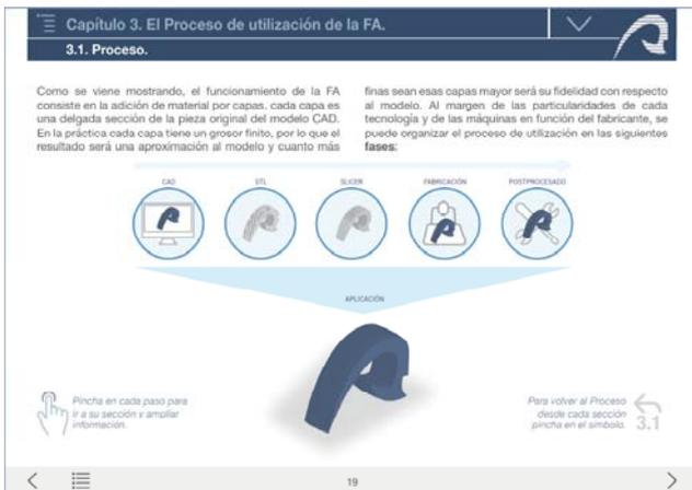
**Figure 16** AM process linked to each stage of its process. ITM in Spanish.
