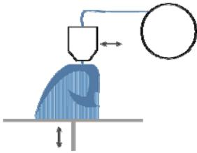
**Figure 5.** Material Extrusion
