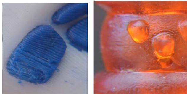
Figure 12. Poor surface finish because of layers, left, VAT Photopolymerisation part which needs postprocessing (cleaning), right.
