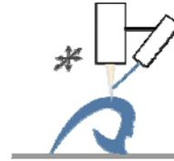
**Figure 9.** Directed Energy Deposition
