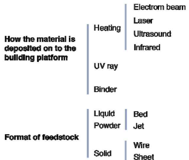
**Figure 2.** Parameters to classify AM techniques or categories.
