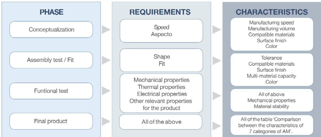
**Figure 14.** First stage of the AM selection process. Designing based on [16].
