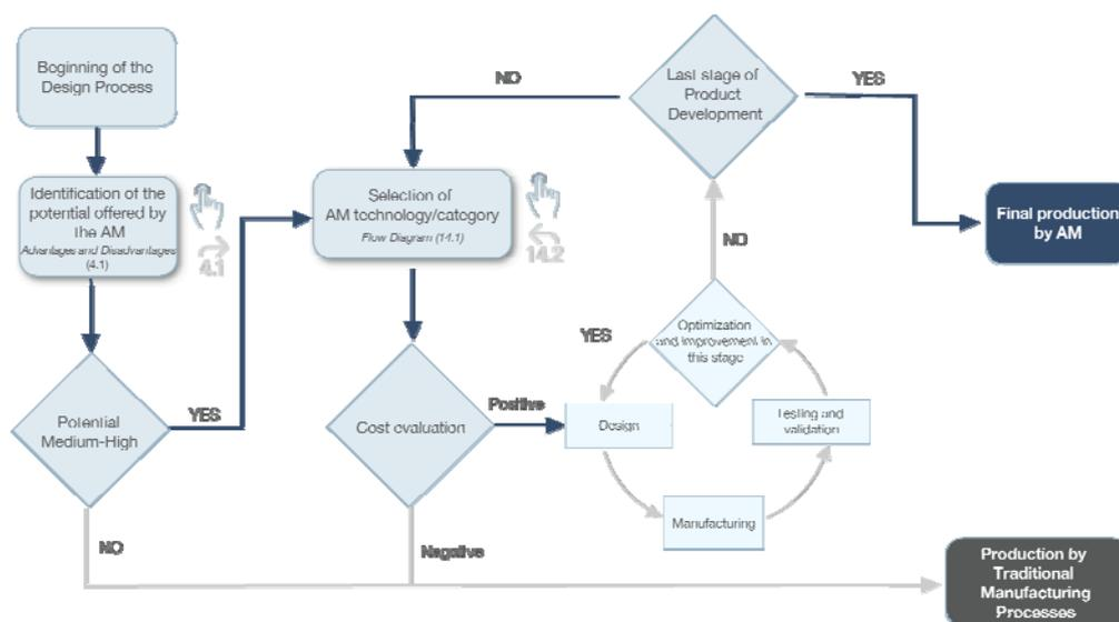
Figure 15. Flow diagram to use AM. Designing based on [15]TM description
