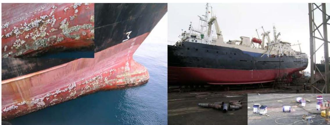
**Figure 1.** Fouling growth, that is, undesirable biological material like algae and barnacles reduces navigability of ships (left picture). The use of antifouling paints, instead, prolongs conservation and facilitates movement of ships (right picture).
