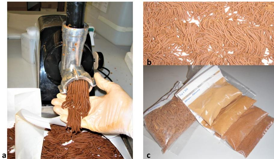
**Figure 21(a, b, c).** a) Compressing processes of the paste; b) compressed paste; c) grounded pellets in sizes.
