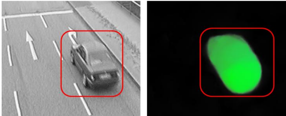
Figure 2.3: Example of motion contours. We see in the image at the right a representation of the flow edges of a moving car by using the IPOL color scheme.
