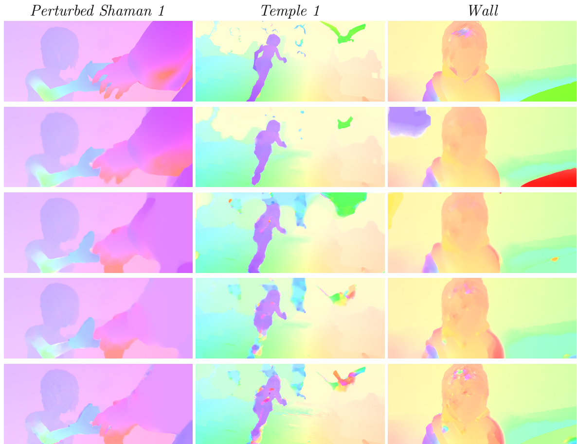
Figure 5.32: Comparison of several optical flow methods using the Sintel Clean test dataset. From top to bottom: The ground truth of three sequences and the results obtained with EpicFlow [Revaud15], LDOF [Brox11b], IPOL-Brox [Sánchez13b] and DF-Auto , respectively
