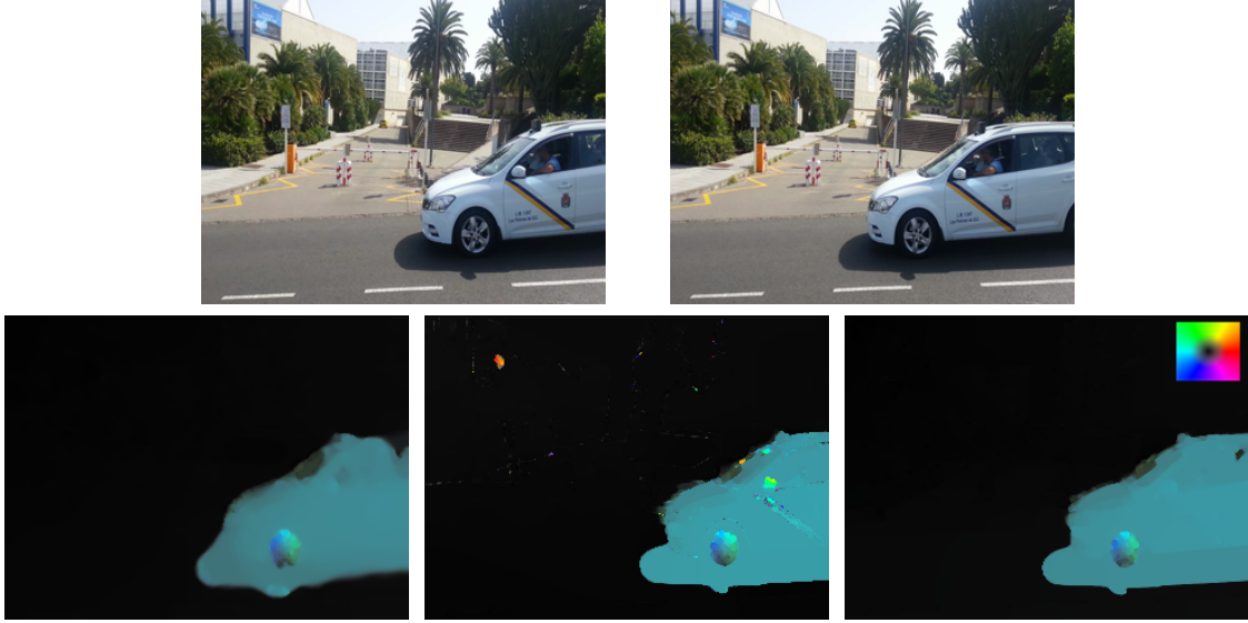
Figure 5.1: Instabilities problem. Top row: first and second frames of a sequence of a moving taxi. Bottom row: first column, the solution obtained with the Brox et al. method; second column, the optical flow obtained with a discontinuity-preserving strategy (note the instabilities that appear in some parts of the motion field); third column, the solution obtained with a similar technique that deals with this type of instabilities.
