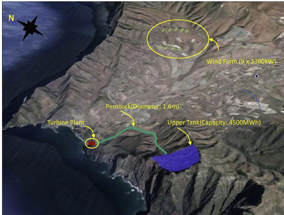
Fig. 15. General layout of the wind-hydro system.
