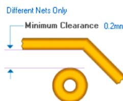
Figura 86. Electrical clearance
