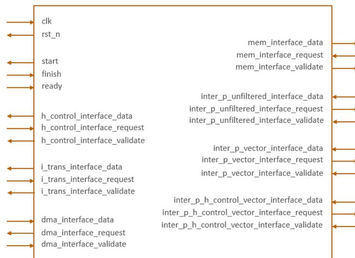
Figura 4.5: Puertos E/S del *testbench*
