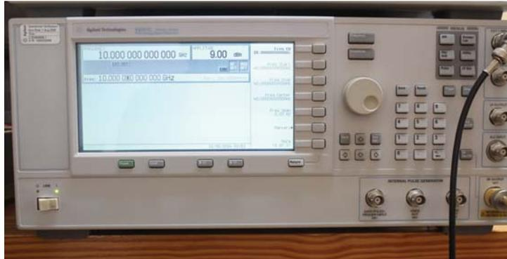
Figura 22 – Generador Agilent Technologies E8257D
