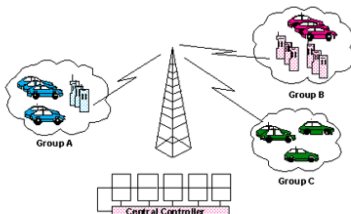
Figura 8: Infraestructura radio trunking.
