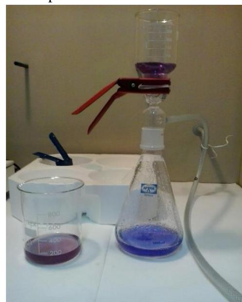
Figure 6. Vacuum system used to filter the water sample.
