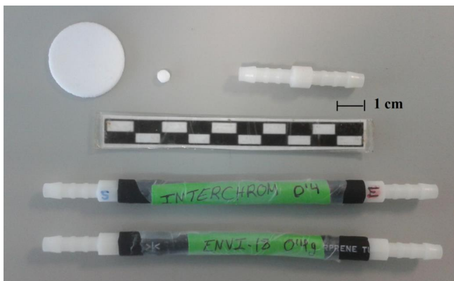
Figure 4: Example of used extraction system, including the internal components added.
