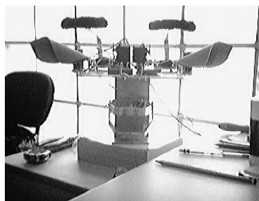
Figure 4: Mechanical structure of the robot head.
