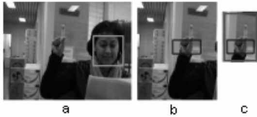
Figure 2. Hand location process: a) face detection, b) wrist detection in the reduced search area, and c) region growing according to general wrist-hand properties.
