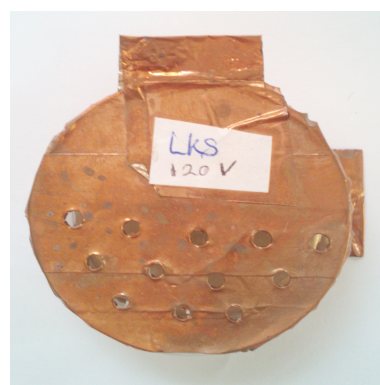
Figure 5. Top of the crystallizer made with a petri dish covered by adhesive copper. In this picture the holes are only placed over the half of the plate. The dimensions of the dish are 6 cm in diameter and 1.5 cm in deep.
