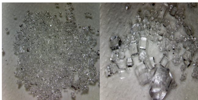
Figure 4. Comparing between the growth obtained without any electric field (left) and an applied one of 4000 V/m (right). It can be notice a variation on the number and size of the crystal which were obtained.
