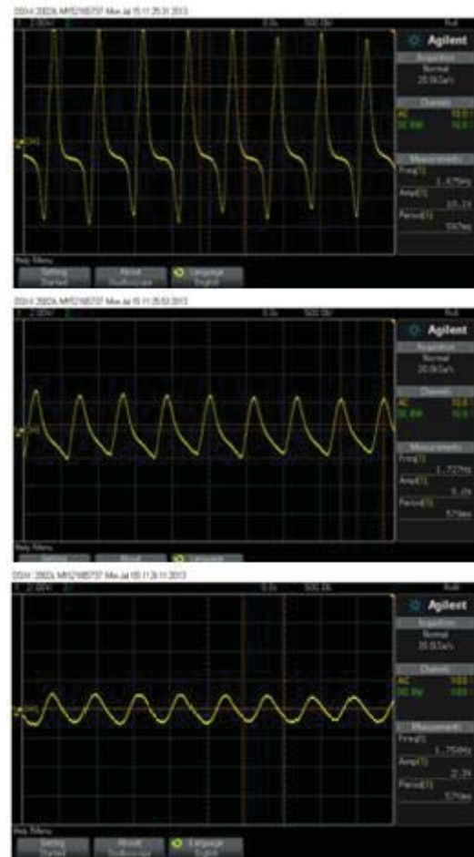
Fig. 3. Signal obtained in the oscilloscope for harmonic and anharmonic oscillations of a pendulum of length 30 cm. These signals are slowly changing with time as the amplitude of the movement is damped.
