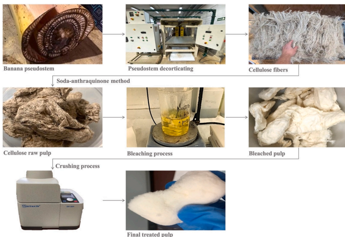
Fig. 1. Mechanical and chemical processes for obtaining cellulose pulp from banana pseudostem.
