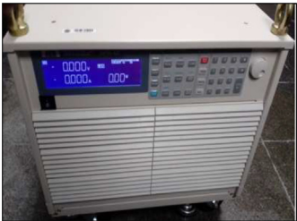
Fig. 6. Adaptive Power 5VP06-42C programmable electronic load used for discharging.
