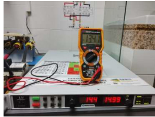
Fig. 3. Magna Power SL100-15/UI programmable DC power supply used for charging.
