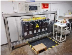
Fig. 7. Experimental bench consisting of six 1200 Ah, 2 V OPzS lead-acid stationary batteries.
