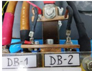
Fig. 4. Protection system with parallel power-blocking diodes.
