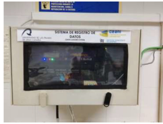
Fig. 2. DataTaker DT85M data logger connected to the acquisition system.
