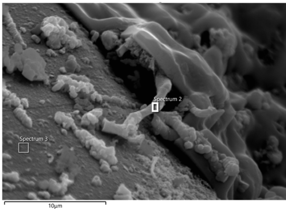
Figure S4. SEM image showing the locations of Spectrum 2 (twisted filament) and Spectrum 3 (chimney surface) used for chemical composition analyses (see Table S5 ).
