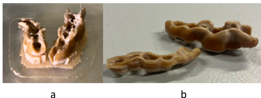
Figure 5. Surgical guide manufactured by MEX: just manufactured (a) and post-processed (b).
