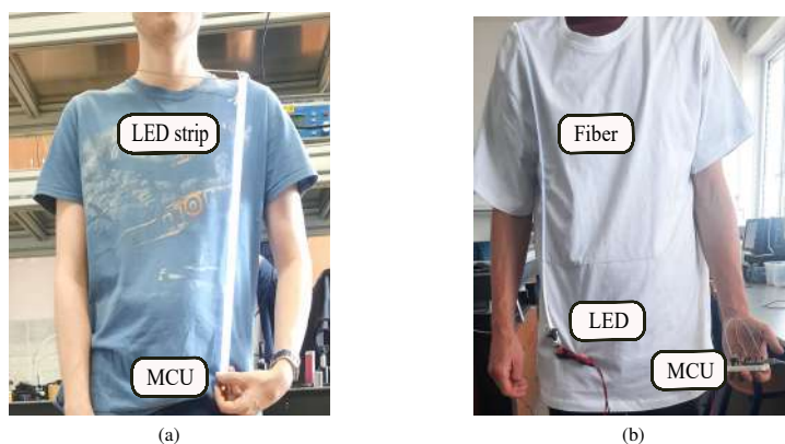
Fig. 3. Wearable experimental setup. (a) LED strip. (b) LED-coupled side-emitting fiber.
