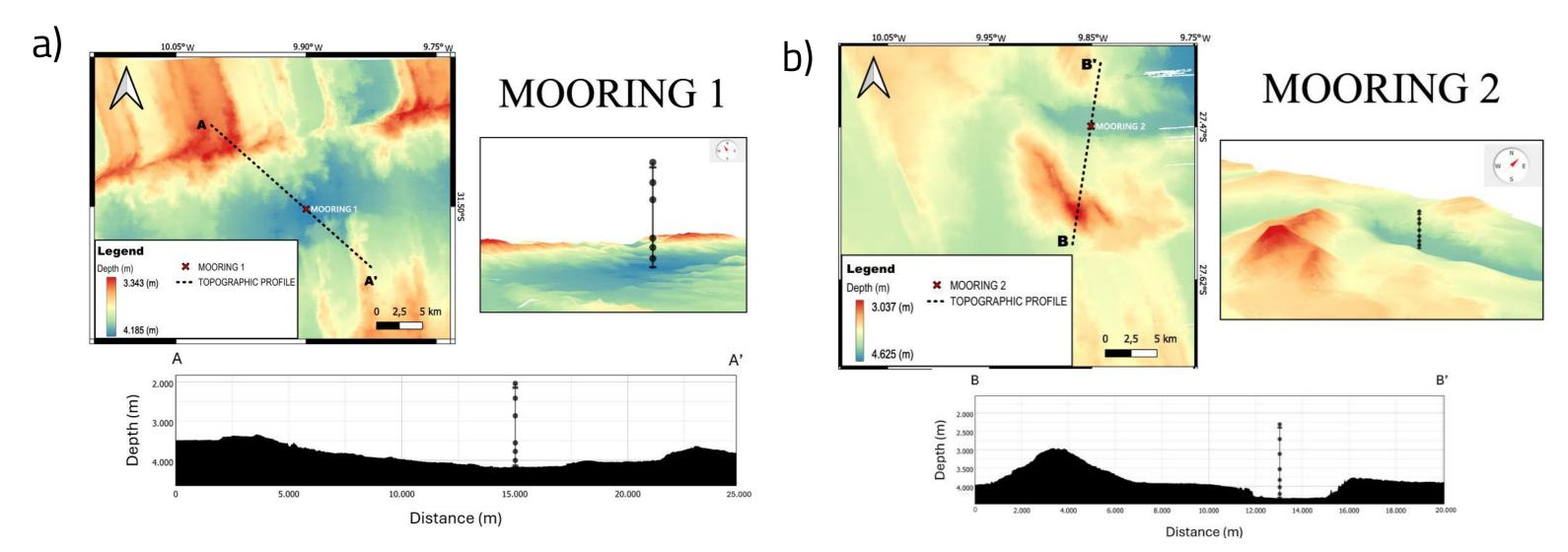
Figure 2. Map showing the locations of Mooring 1 (a) and Mooring 2 (b). It includes a 3D composition and a topographic profile that illustrates the orography of installation area. Additionally, the mooring line and the instruments are scaled to the image, with current meters represented as spheres and MicroCATs as rectangles.
