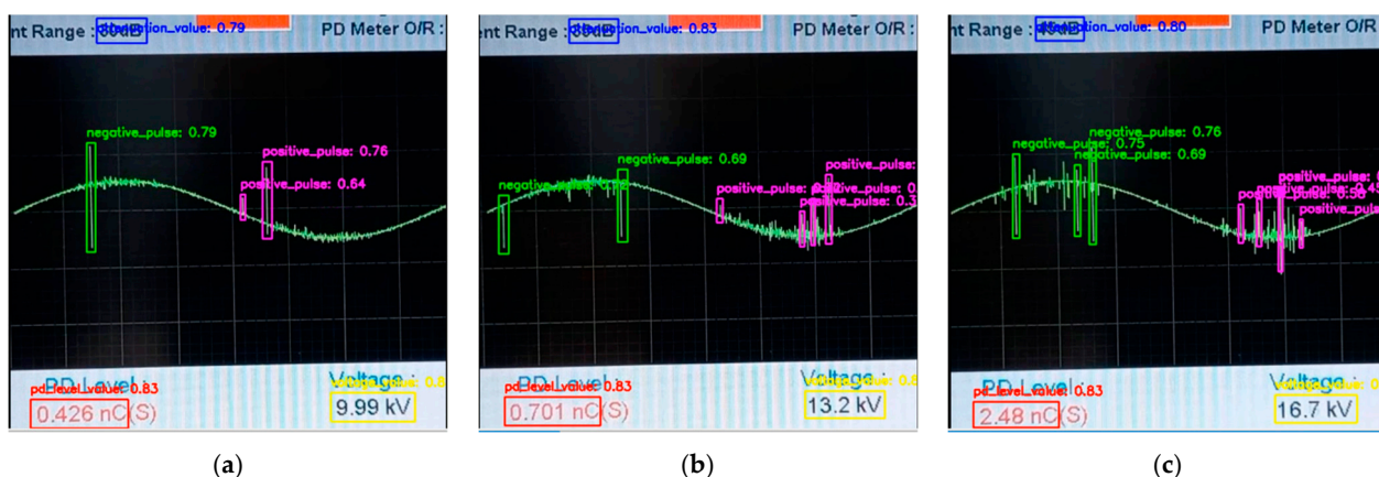
Figure 16. Inference for 3 images from the trained CNN. (a) PD detection for 10 kV. (b) PD detection for 13 kV. (c) PD detection for 16 kV.
