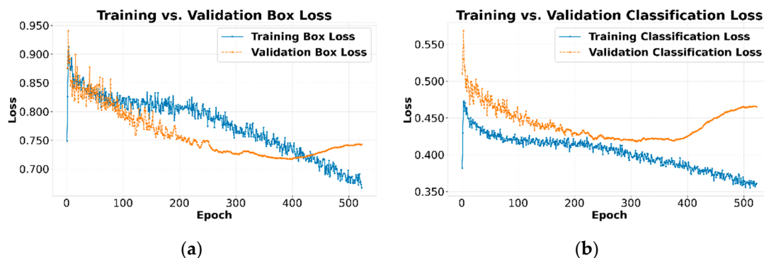
Figure 20. Training vs. Validation Box and Classification curves. (a) Training vs. Validation Box Loss. (b) Training vs. Validation Classification Loss.
