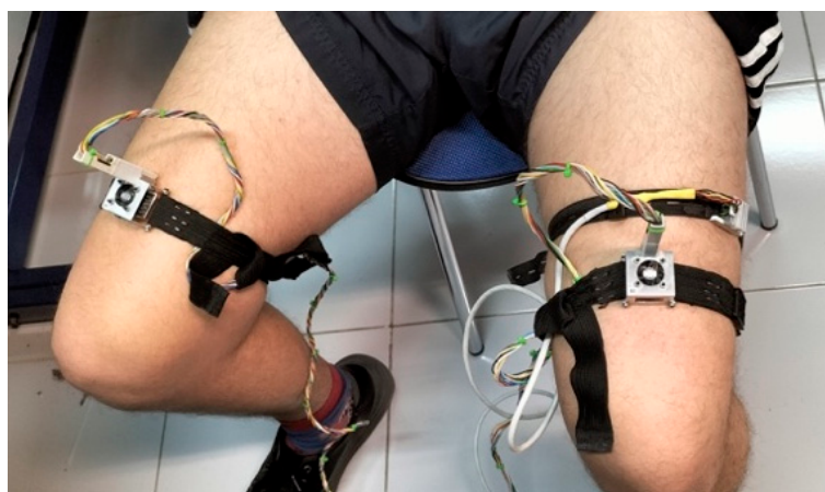
Figure 4. Placement of the skin calorimeters for the measurement of skin thermal properties.
