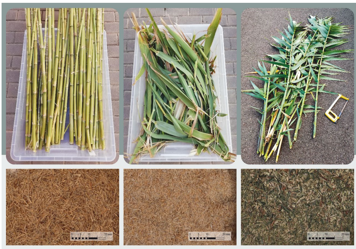
Figure 3. Fibres obtained from Arundo donax L. culms, leaves and whole plants (from left to right).
