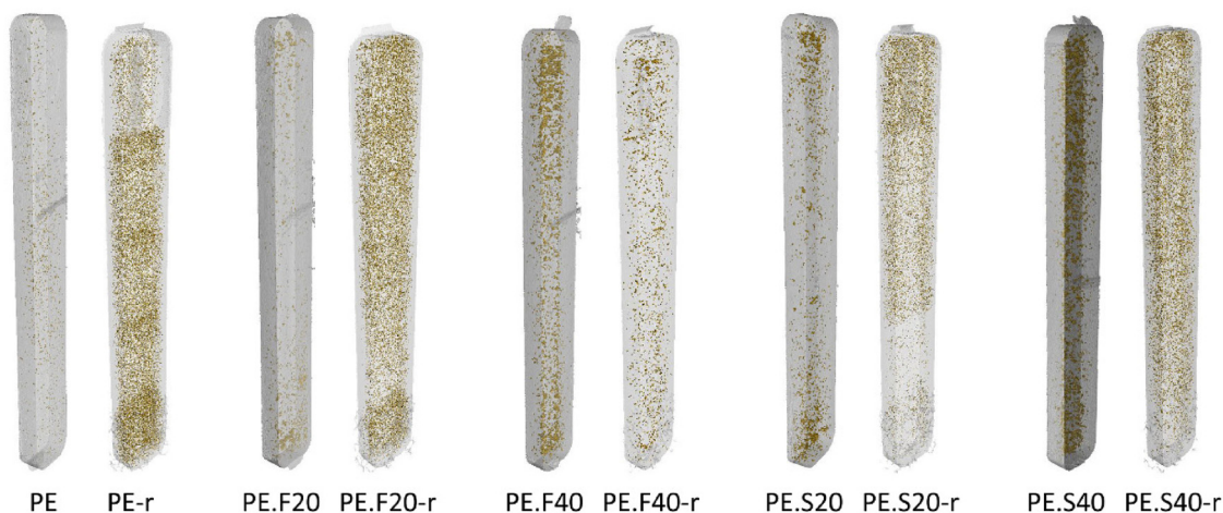
Figure 15: 3D computed tomography images presenting pores distribution.
