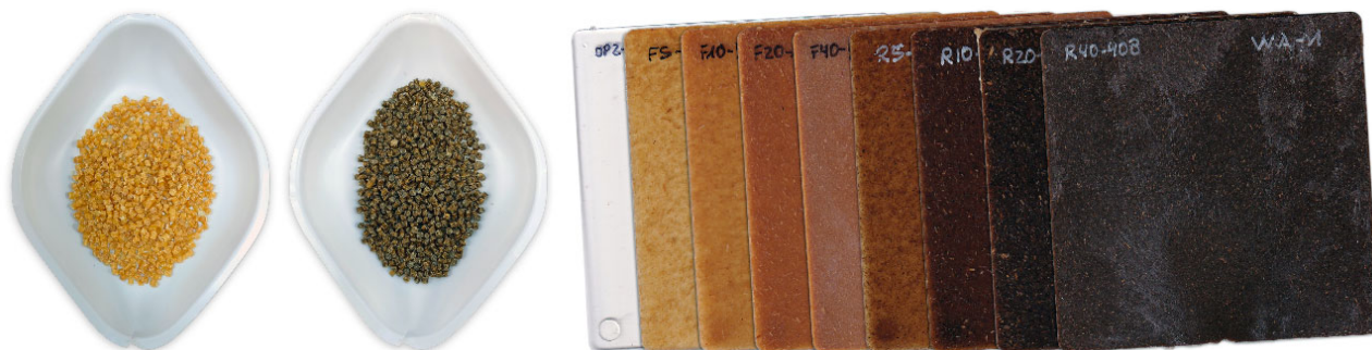
Figure 2. Extruded compound (PLA.F20 and PLA.S20) and injection moulded plates (all formulations).
