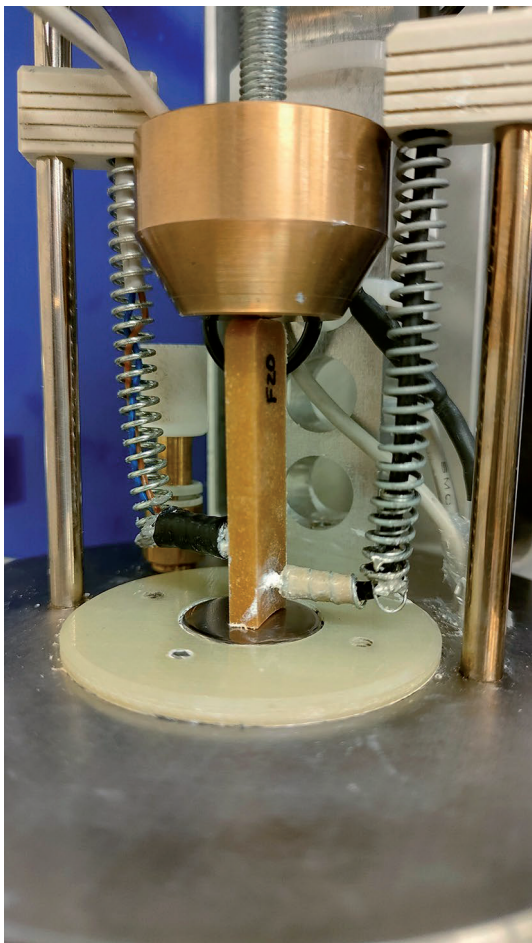
Fig. 1 Experimental setup for the measurement of thermal diffusivity
