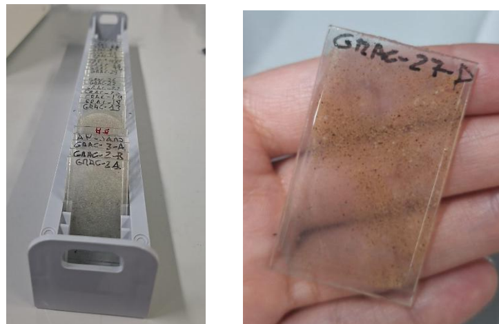
Figure 6. Images of the thin sections to which the petrographic study was carried out. In the right photograph, there is a thin section of sands and silts cemented with epoxy from an endorheic basin of Salado beach, La Graciosa, which were used for the petrographic study.
