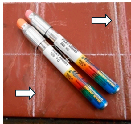
Figure 3. Markal Thermomelt heat sticks, used as a backup method, allow for broader use but are less defined, the arrows show the thermal wax lines parallel to the more defined chalk ones.
