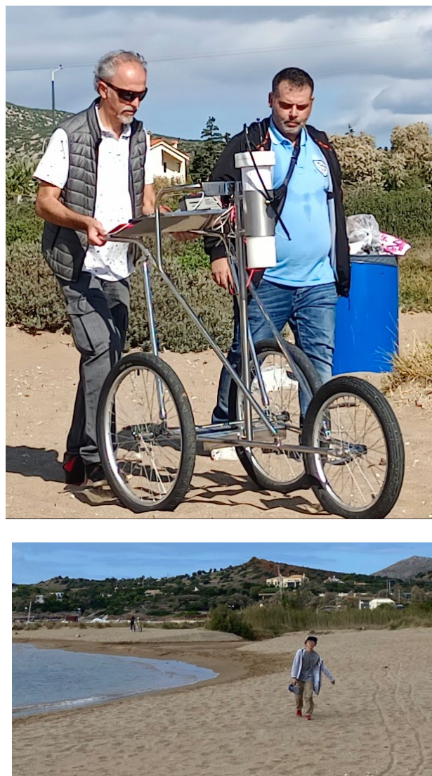
Figure 2. The trolley configuration where the KATERINA II geo-referenced detection system is installed together with the other modules ( upper photo ) and a surveyor carrying a MEDUSA sensor ( lower photo ).
