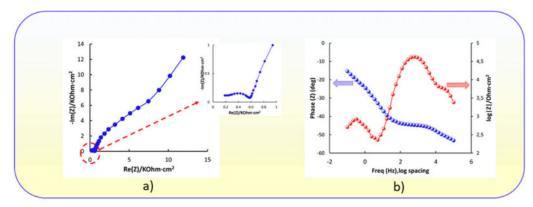
Fig. 4. Impedance diagrams: a) Nyquist; b) Bode-IZI and Bode-phase, for dopped sample in 3.5% NaCI
