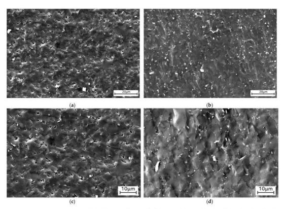
Figure 2. SEM images of (a) monolithic  $B_4C$  at  $3500\times$  magnification, (b) 3% HEA-doped  $B_4C$  at  $3500\times$  magnification, (c) monolithic  $B_4C$  at  $5000\times$  magnification, and (d) 3% HEA-doped  $B_4C$  at  $5000\times$  magnification.
