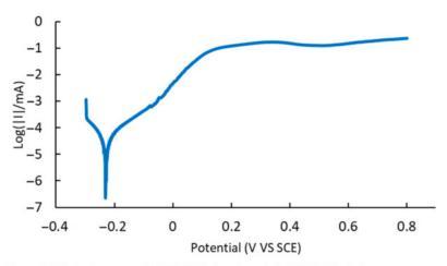
Figure 4. Polarization curve of B<sub>4</sub>C 3% HEA-doped sample in 3.5% NaCl solution.
