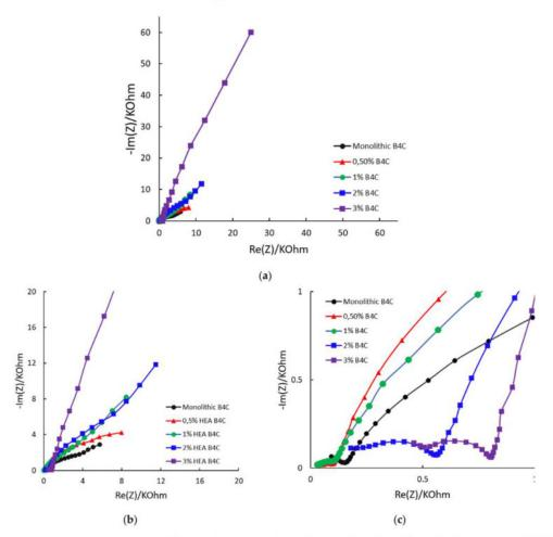
Figure 7. Nyquist diagrams for the studied samples at  $E_{corr}$  after 24 h of immersion in 3.5% NaCl solution: (a) complete plot; (b) detail at medium frequencies; (c) detail at low frequencies.
