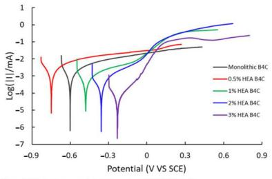
Figure 4. Polarization curve of studied samples in 3.5% NaCl solution.
