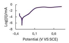
Fig. 1. Linear polarization Rate of doped B<sub>4</sub>C sample.
