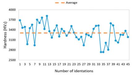
Figure 8. Microhardness values of each indentation for B<sub>4</sub>C 3% HEA sample.
