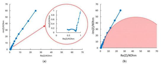
**Figure 6.** Nyquist diagrams for doped samples at Ecorr after 24 h of immersion in 3.5% NaCl solution with (a) higher detail at low frequencies and (b) higher detail at medium frequencies.
