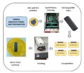
Figure 1. Schematic representation of the material preparation.
