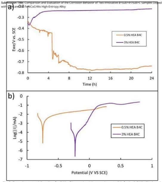
Fig. 2. Corrosion potential vs. time for 24 h of immersion (a)), corrosion rate (b)), for both B4C HEA-doped samples in 3.5% NaCl solution.
