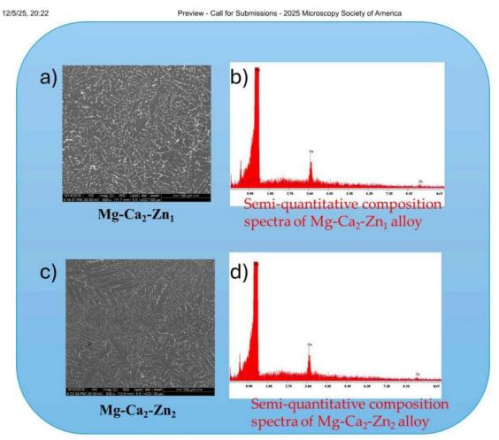
Fig. 2. SEM microstructure of Mg-Ca-Zn alloys.
