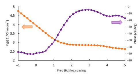
**Figure 5.** Bode-IZI and Bode phase for doped samples at Ecorr after 24 h of immersion in 3.5% NaCl solution.
