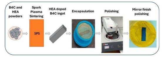
Figure 1. Schematic representation of the material preparation.
