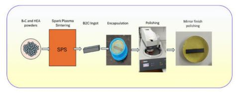
Fig. 1. Sample manufacturing process and preparation.
