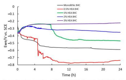
$\textbf{Figure 3.} \ Comparison \ of corrosion \ potentials \ vs. \ time \ for \ 24 \ h \ of \ immersion \ in \ 3.5\% \ NaCl \ solution \ of \ studied \ samples.$
