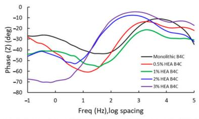
Figure 6. Bode phase for the studied samples at E<sub>corr</sub> after 24 h of immersion in 3.5% NaCl solution.
