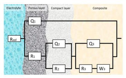
Figure 7. Equivalent circuit R(Q(R(QR)Q(RW))).
