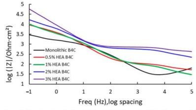
Figure 5. Bode impedance for the studied samples at Ecorr after 24 h of immersion in 3.5% NaCl solution.
