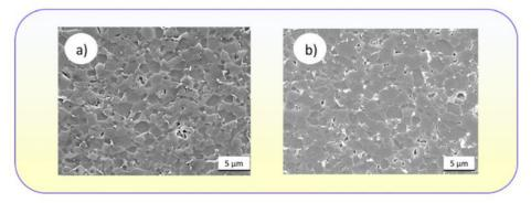
Fig. 2. SEM images of the a) B<sub>4</sub>C ceramic and b) HEA doped ceramic.
