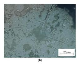
Figure 10. B<sub>4</sub>C doped sample (a) before Vickers indentation and (b) after Vicker indentation.
