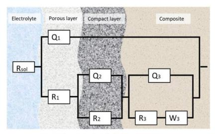
Figure 8. The equivalent circuit for the fitting of the EIS data.
