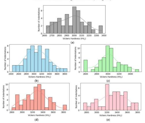
Figure 9. Histogram of Vickers hardness for (a) monolithic  $B_4C$ ; (b) B4C.05; (c) B4C.1; (d) B4C.2; and (e) B4C.3.
