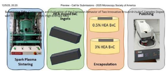
Fig. 1. Fabrication and preparation of the B4C samples under study.
