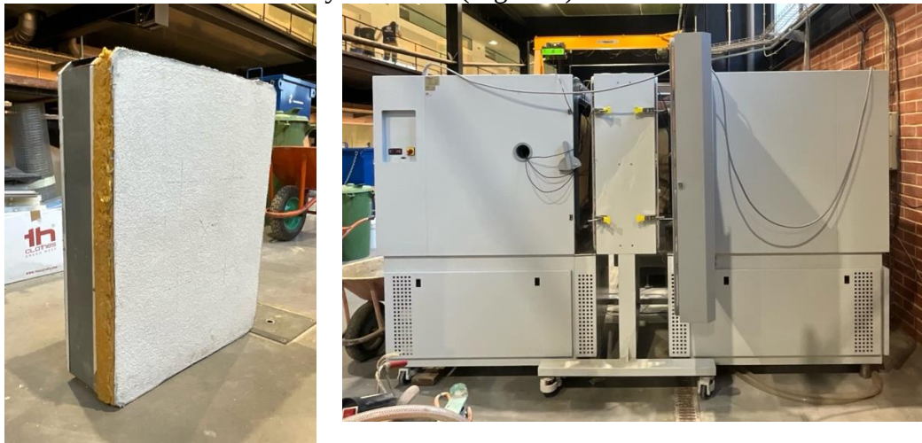
Figure 6. Image of the LSF wall and hot-box equipment.
