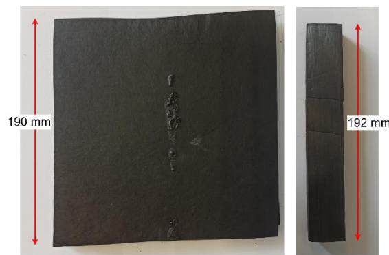
Figure 3. MDF and pine wood samples after being cooled to room temperature.
