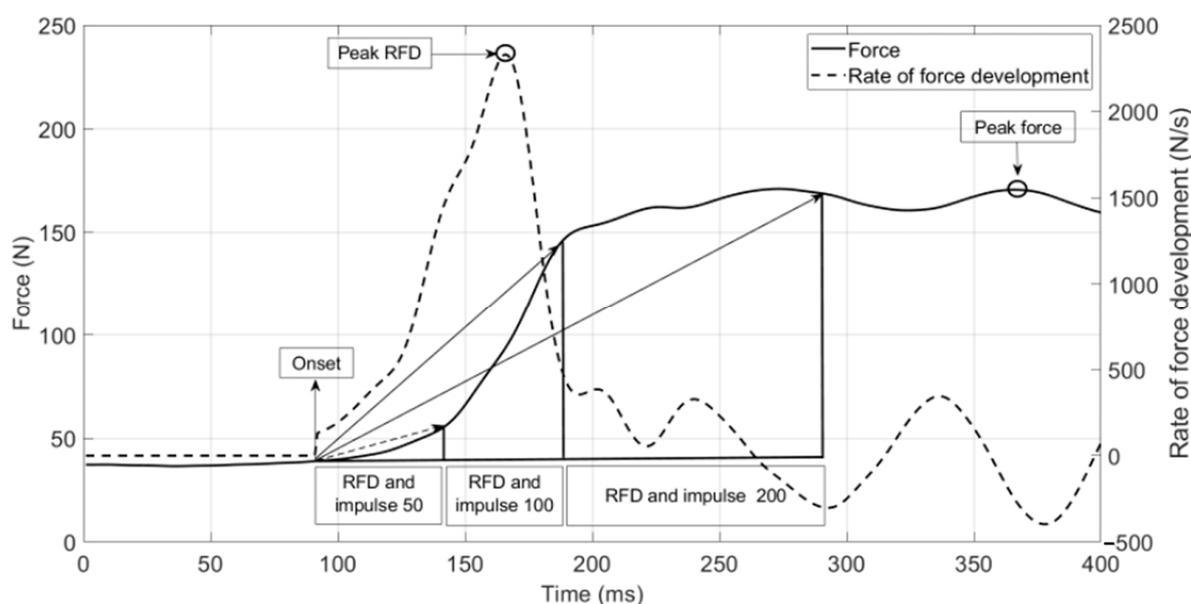
**Figure 2.** Signal shape of force and rate of force development (RFD).
