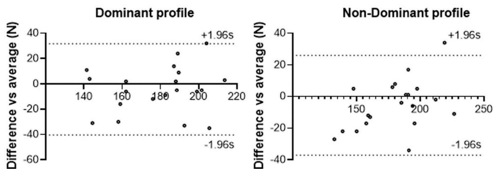
**Figure 3.** Bland–Altman plots of peak force in both profiles. s standard deviation of bias.
