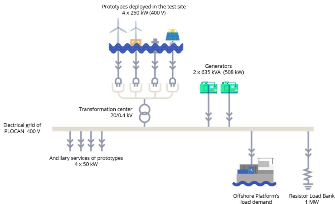
**Figure 6.** Electric diagram of the modelled system according to the current PLOCAN SmartGrid.
