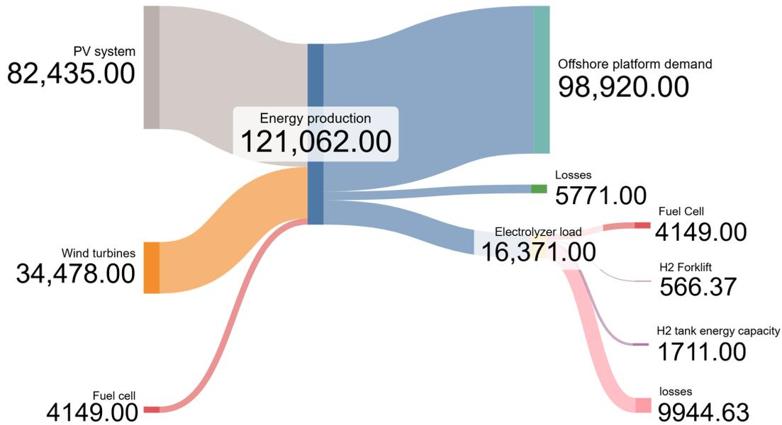
Figure 10. Sankey diagram of the energy balance of the optimized target PLOCAN SmartGrid.
