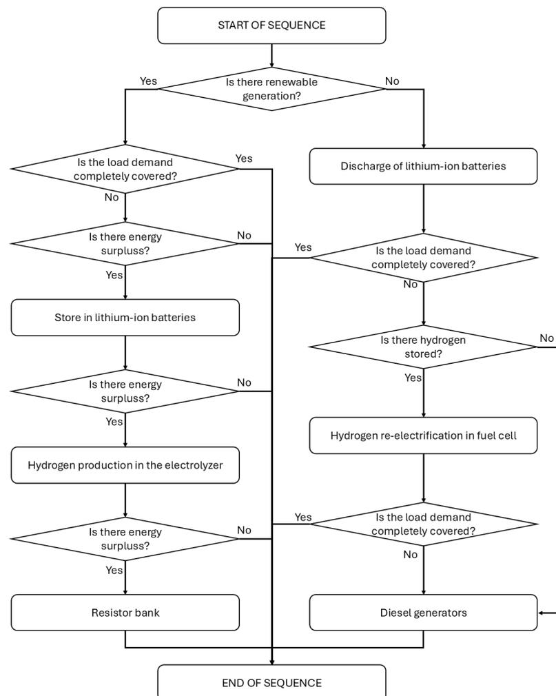
Figure 8. Sequence of operation of the target simulated system.
