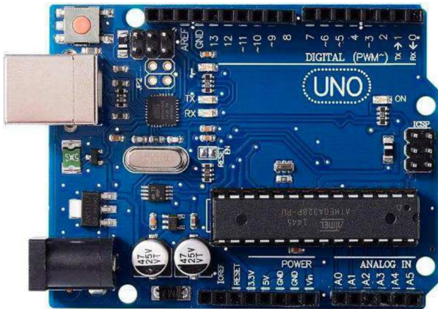
Fig. 4 Plan view of an Arduino UNO-R3 chip. Its components and its motherboard can be seen
