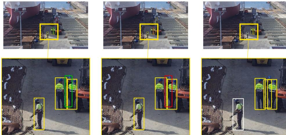
**Fig. 11.** Comparison of the results obtained when workers are close to each other and their bounding boxes overlap: our method (left), Nath's (middle), and Xiong's (right). For each method: result for the whole scene (top), and enlargement of the selected area (bottom).
