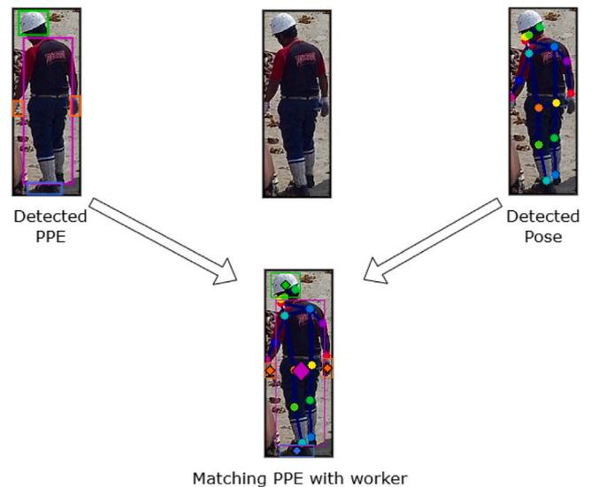
Fig. 3. Worker-PPE matching: in each cropped image (top middle), PPE is detected (top left) and pose is estimated (top right). The distance from the center of each PPE element (colored rhombi) to the corresponding body part (colored circles) is used for worker-PPE matching (bottom).
