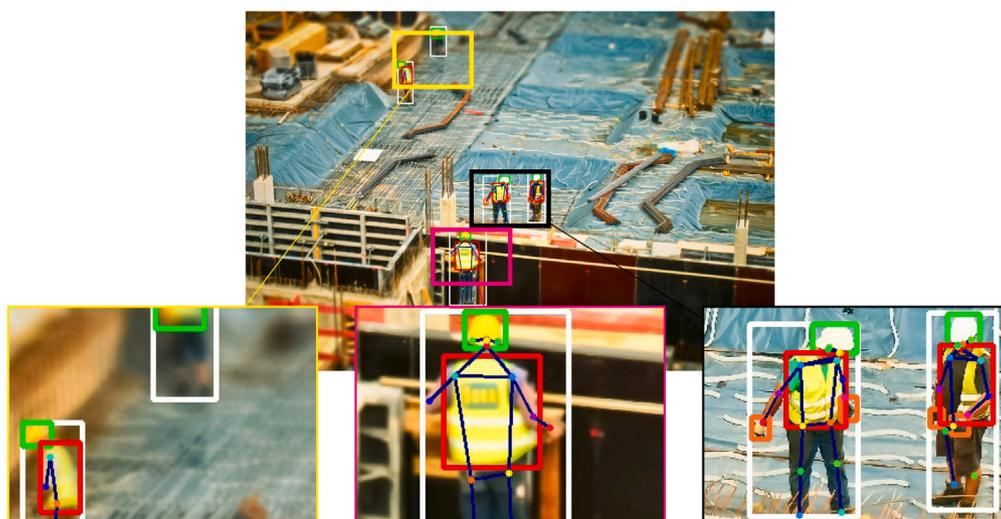
Fig. 5. Results for worker and PPE detection and matching in challenging scenarios: long distance. Whole scene (top) and enlarged areas (bottom).
