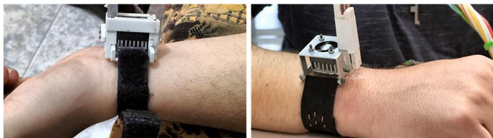
**Fig. 10.** Calorimeters  $S0$  and  $S1$  placed on the dorsal and volar areas of the wrist.
