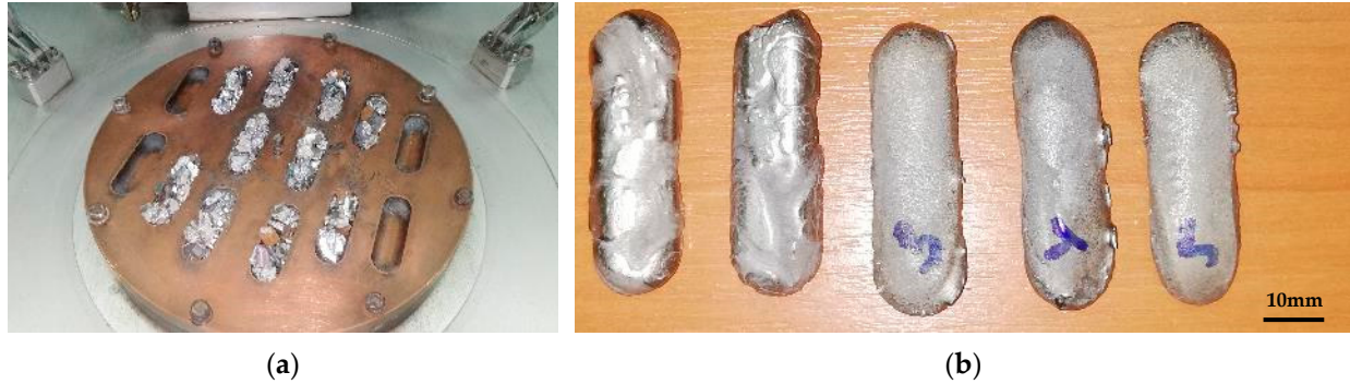
Figure 1. (a) The metallic load placed on the copper plate of the VAR equipment and (b) FeMoTaTiZr mini-ingots of high-entropy alloy obtained by melting in RAV.
