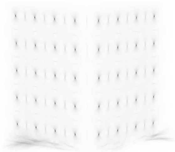
Figure 5: Gray level image representation of the accumulator. White regions represent less voted pixels and black regions are the most voted ones
