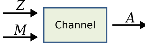
Figure 6.5: Channel of two inputs. Using the reference of the CLHU, the ‘bottleneck’ information transmission is carried out by two channels AZ and AM .
