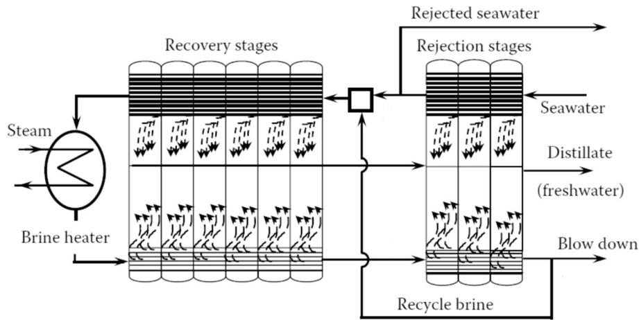
Fig. 3. A representation of the brine recycling MSF process (Adapted from [29]).
