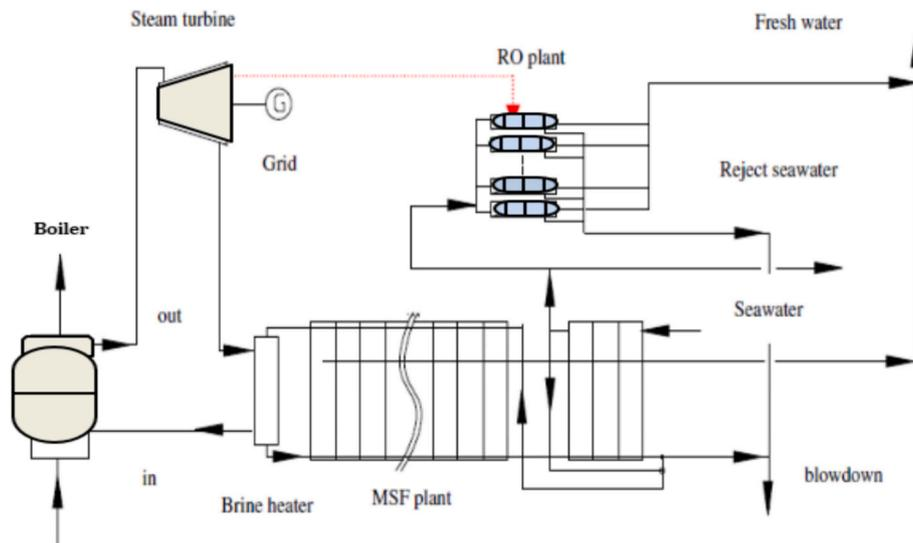
Fig. 14. A representation of the cogeneration system of the power plant/RO-MSF hybrid system (Adapted from [45]).
