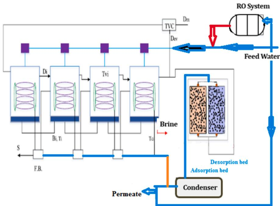
Fig. 23. A representation of the RO-MED/TVC hybrid system with adsorption unit for seawater desalination (Adapted from [54]).
