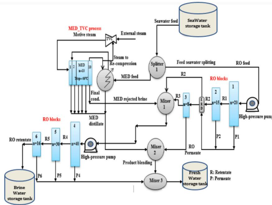
Fig. 29. A representation of integrated system of double permeate and retentate reprocessing RO modes and MED unit for seawater desalination (Adapted from [58]).
