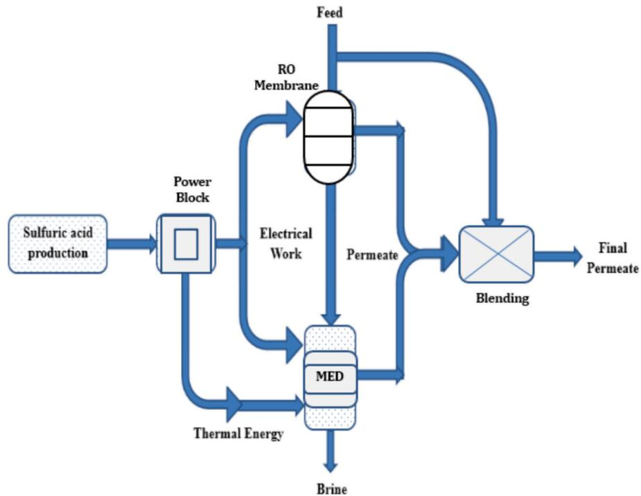
Fig. 25. An integrated system of RO and MED with heat recovery from sulfuric acid production unit (Adapted from [56]).
