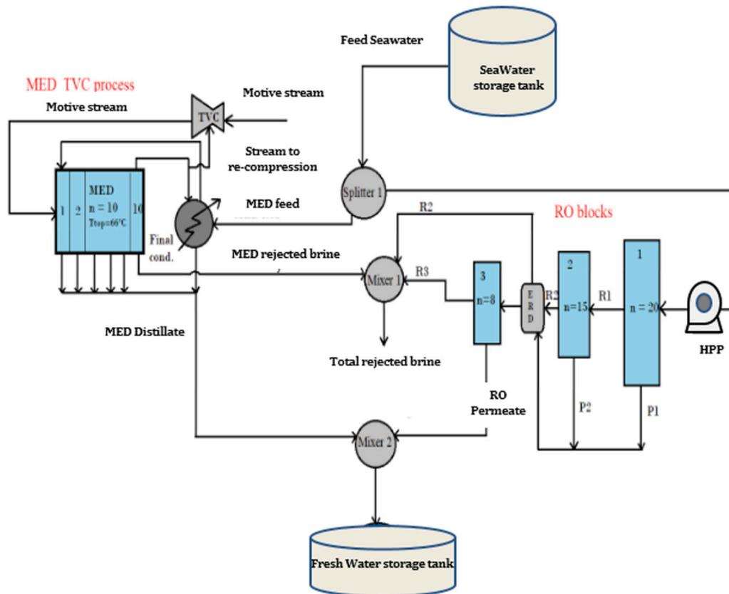
Fig. 24. A representation of integrated permeate reprocessing RO and MED/TVC units (Adapted from [55]).
