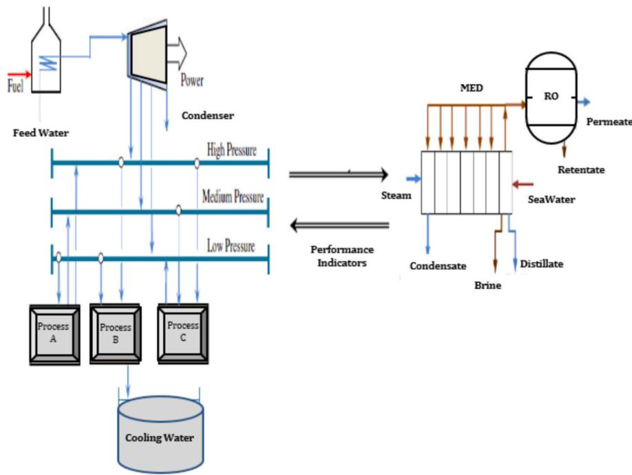
Fig. 18. A representation of the RO-MED hybrid system coupled to a steam network of site utility (Adapted from [50]).
