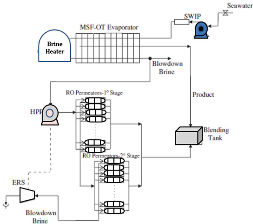
Fig. 10. A representation of integrated RO-MSF systems (Adapted from [42]).
