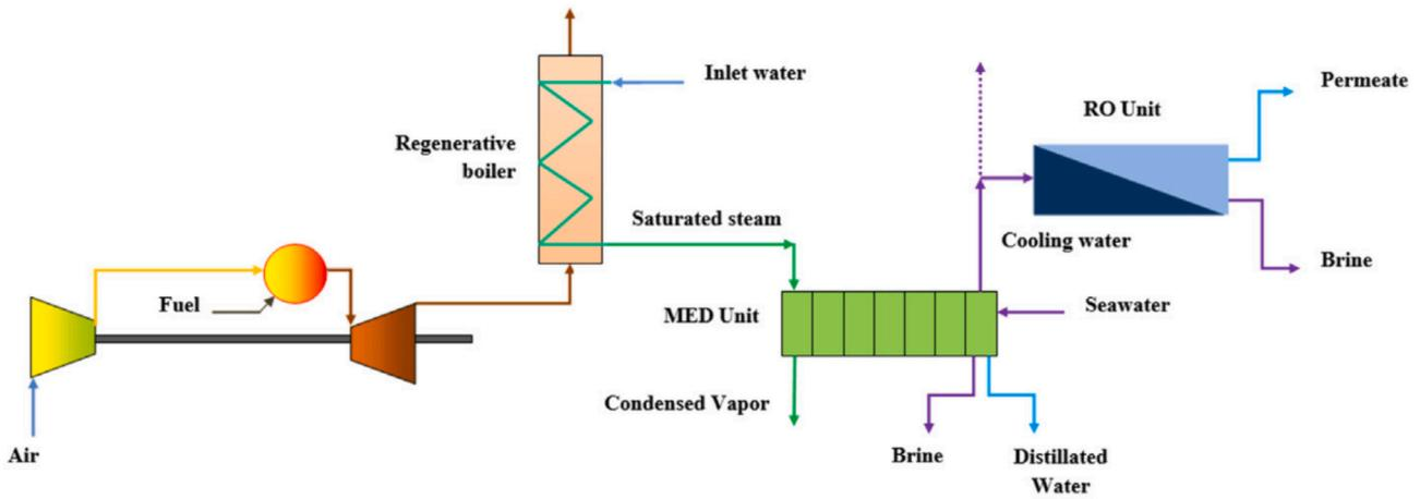
Fig. 30. A representation of the RO-MED system and gas turbine cycle (Adapted from [60]).
