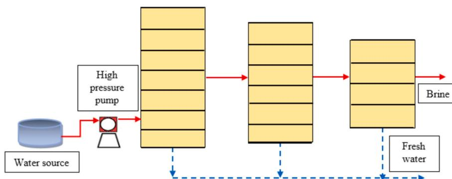
Fig. 2. A simple schematic diagram of a multistage RO process.
