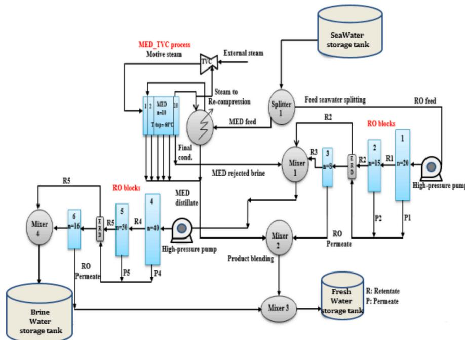
Fig. 28. A representation of double permeate reprocessing RO unit and MED unit for seawater desalination (Adapted from [58]).
