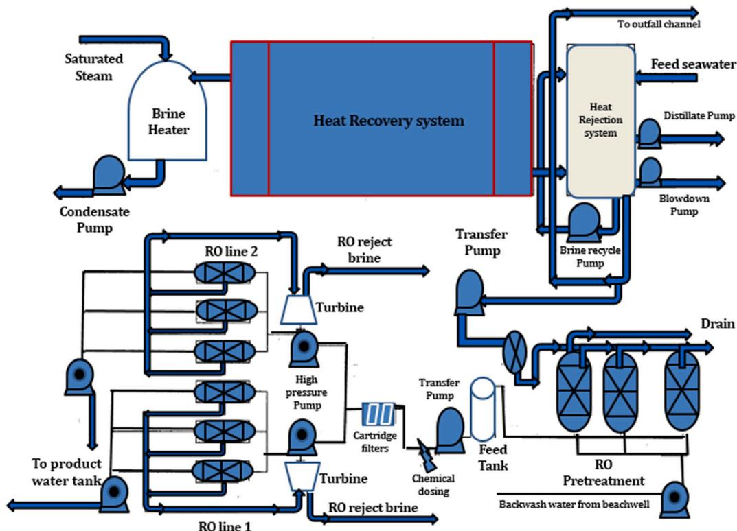
Fig. 6. A representation of an integrated RO-MSF system (Adapted from [36]).
