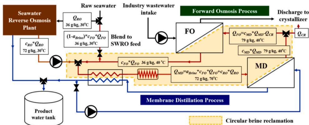
Fig. 32. SWRO-MD-FO brine reclamation hybrid system flow diagram [82].
