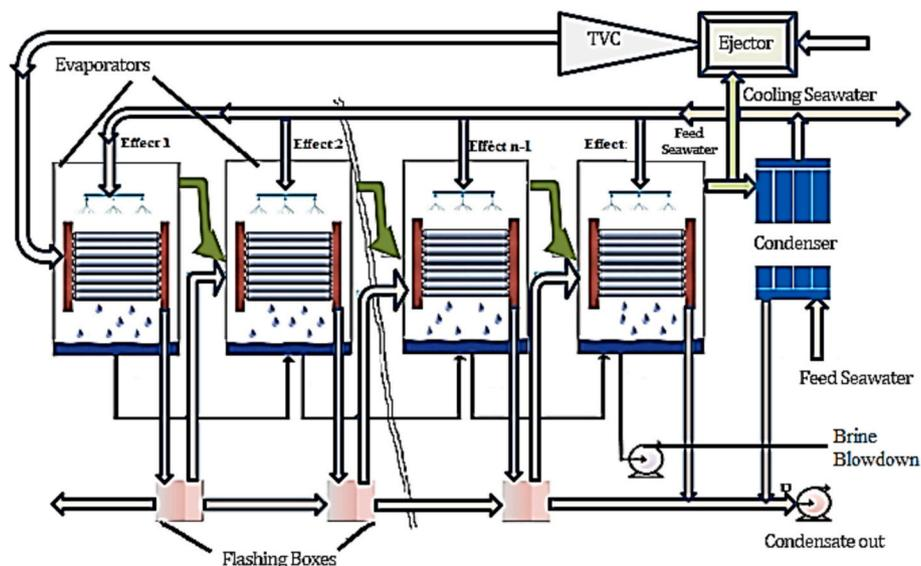
Fig. 4. A representation of MED coupled to TVC process (Adapted from [33]).
