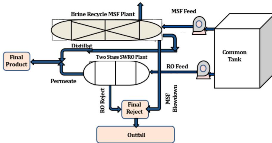
Fig. 8. A representation of an independent two stages RO and brine recycle MSF and common intake (Adapted from [40]).
