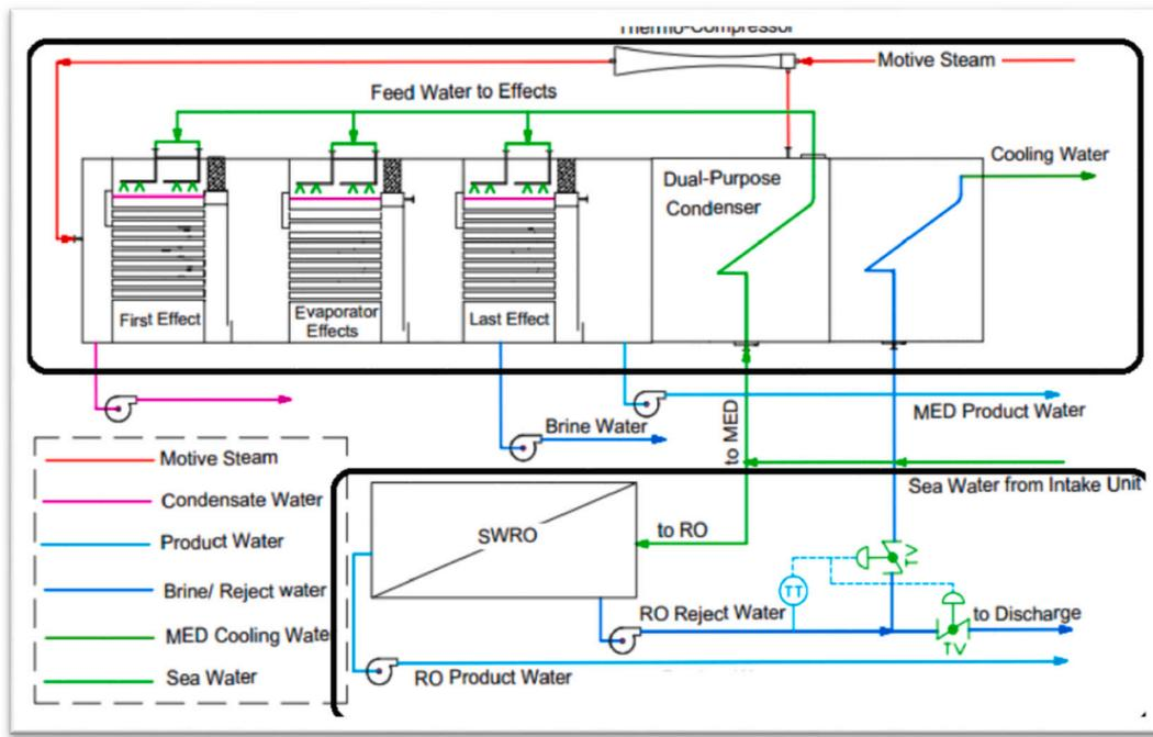
Fig. 27. An integrated system of RO and MED using the second internal coupling technique (Adapted from [57]).
