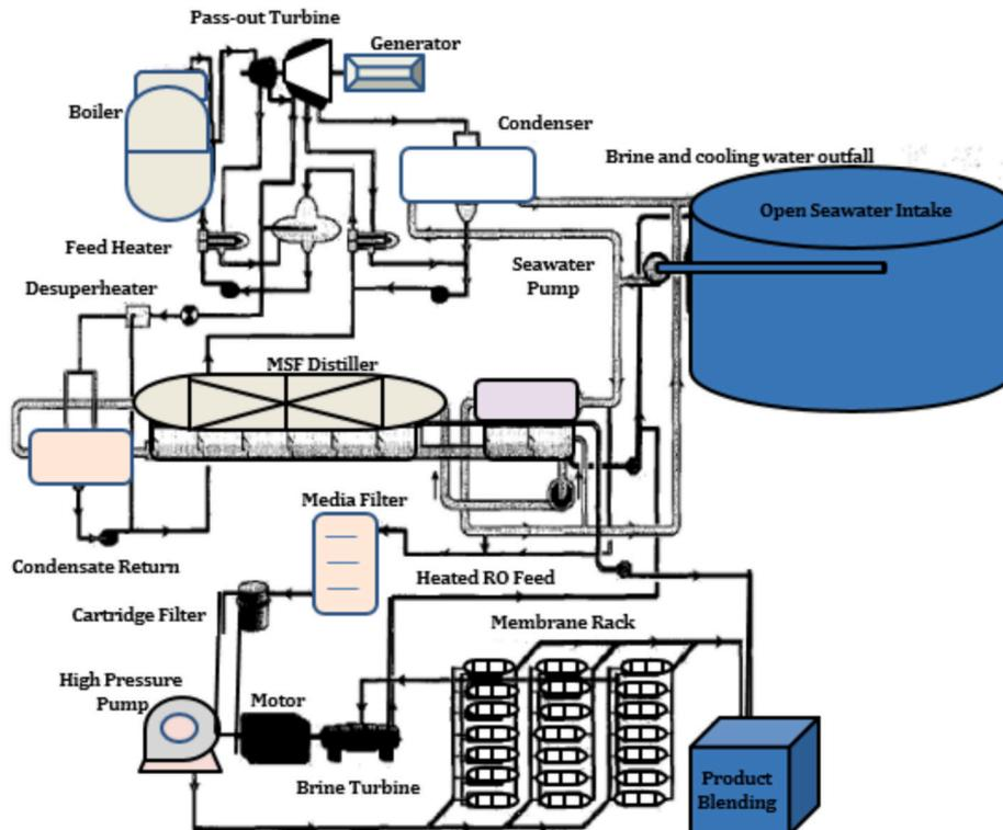
Fig. 7. A representation of the integrated RO-MSF system (Adapted from [37]).
