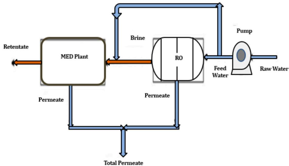
Fig. 20. A representation of the series mode of the integrated RO- MED/TVC units (Adapted from [52]).
