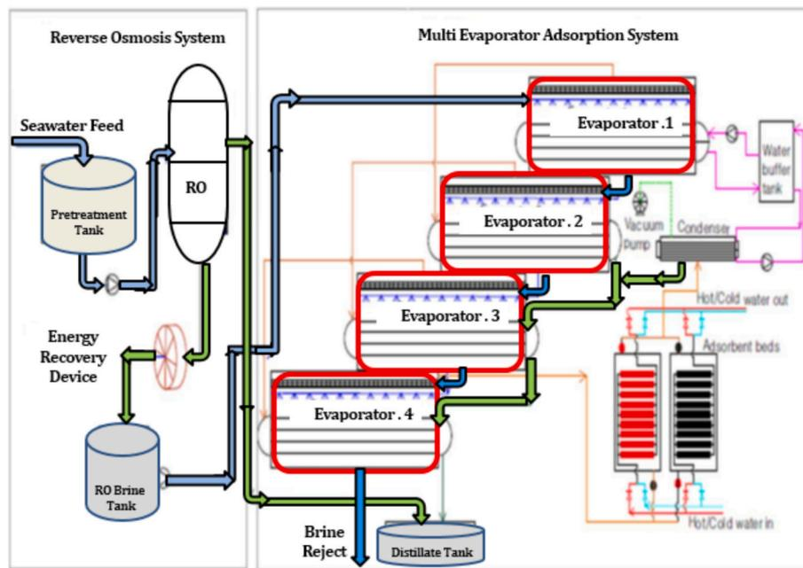
Fig. 19. A representation of RO unit and the multi-evaporator adsorption system (Adapted from [51]).
