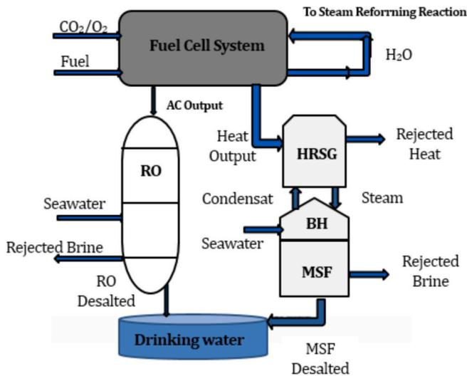
Fig. 11. Integrated fuel cell and RO-MSF systems (Adapted from [43]).
