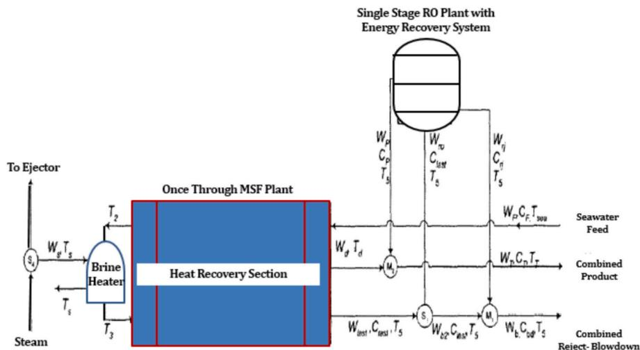
Fig. 9. A representation of a fully integrated seawater desalination plant of once-through and RO processes (Adapted from [40]).
