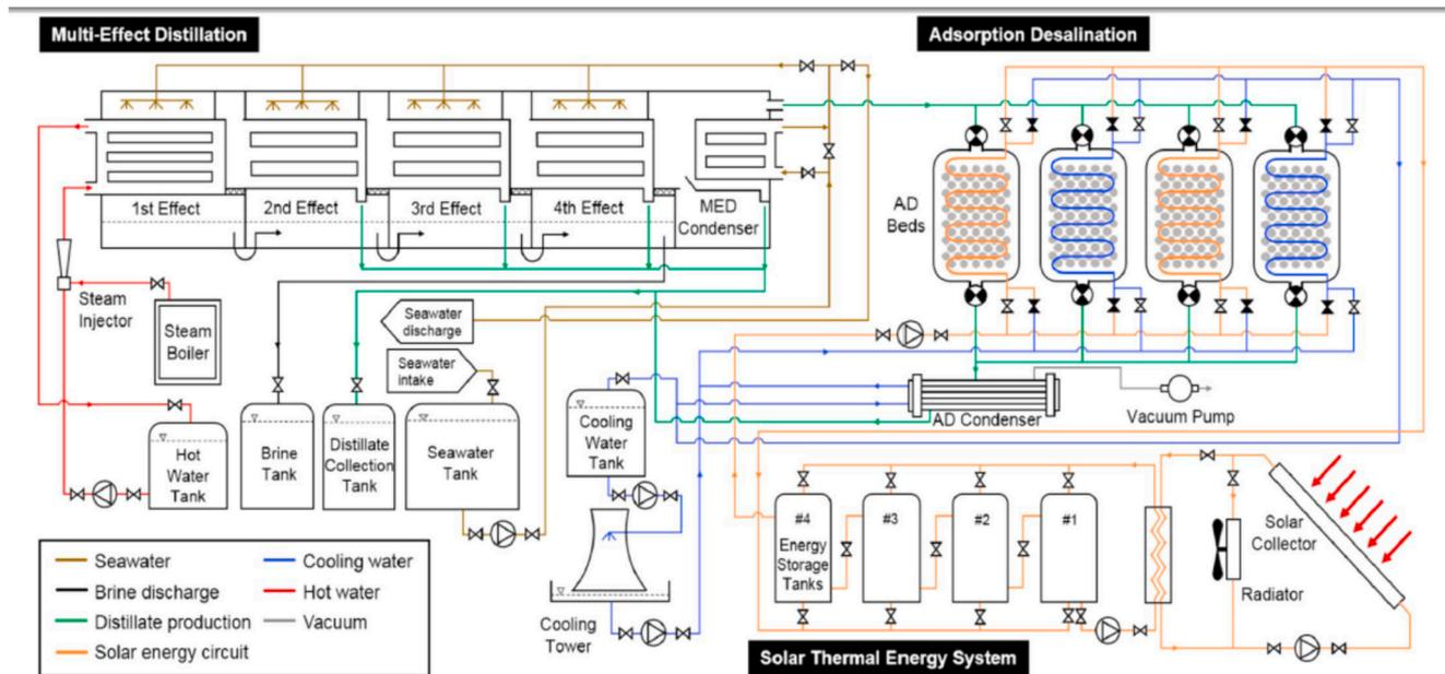
Fig. 35. An integrated system of MED-AD-Solar thermal energy unit [84].
