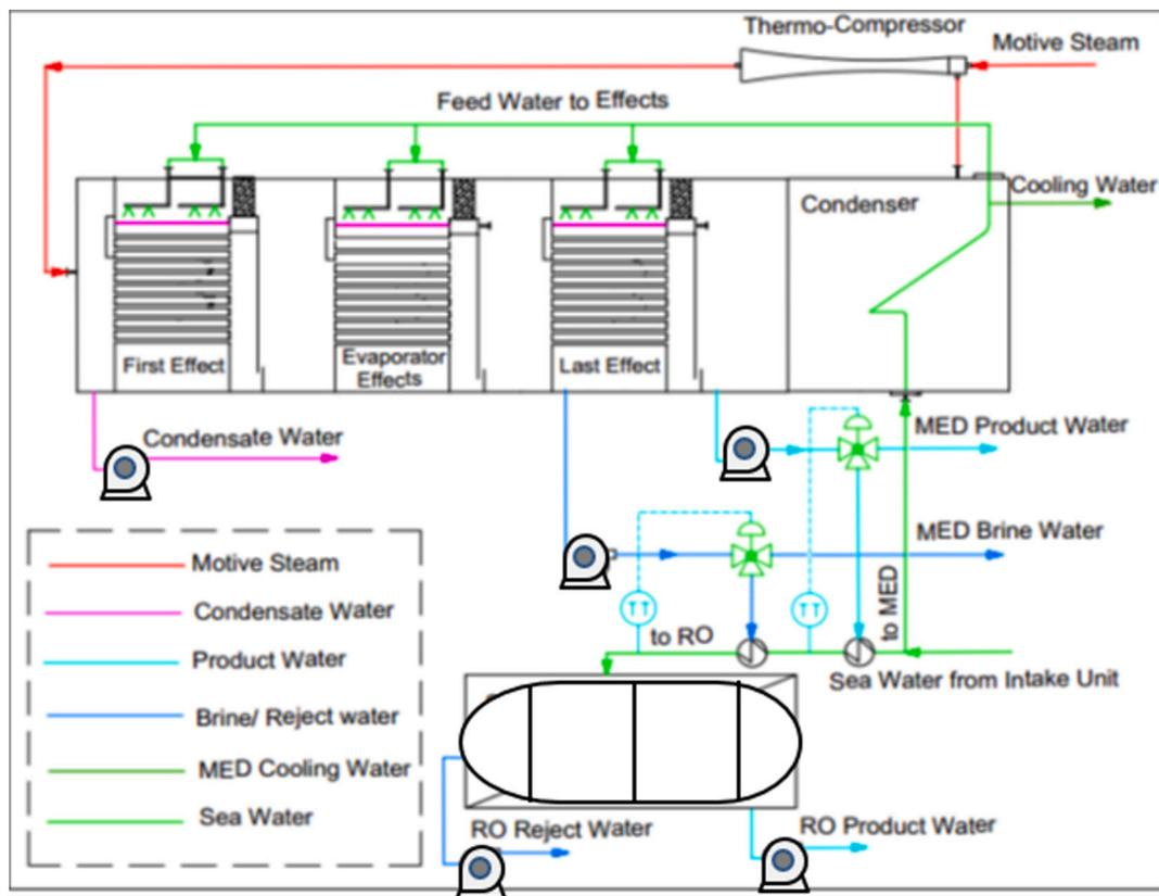
Fig. 26. An integrated system of RO-and MED using the first internal coupling technique (Adapted from [57]).
