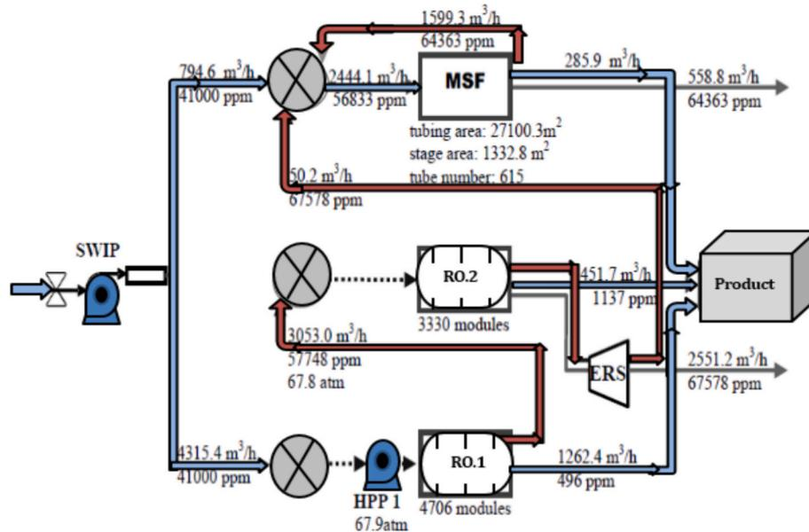
Fig. 13. A representation of the optimal design of two RO units and one MSF unit (Adapted from [44]).
