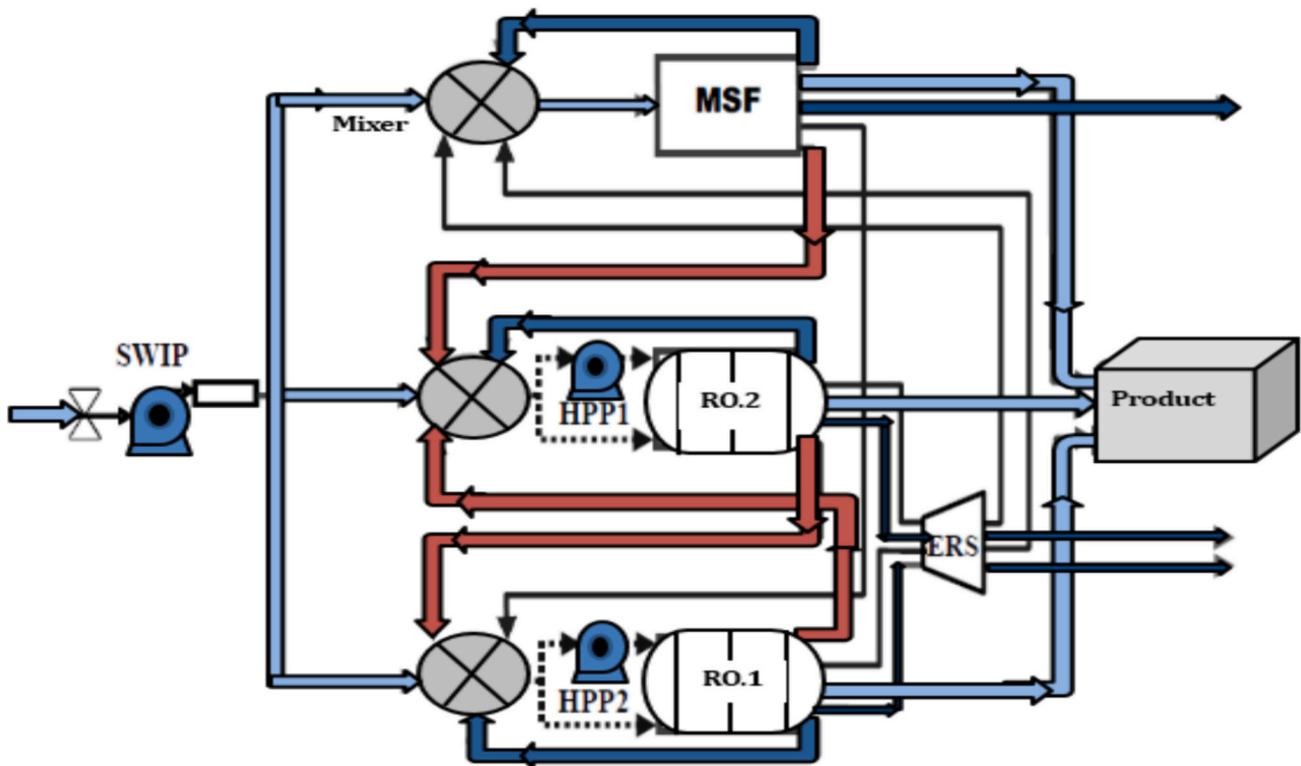
Fig. 12. A representation of the proposed integration of two RO units and brine recycling MSF (Adapted from [44]).
