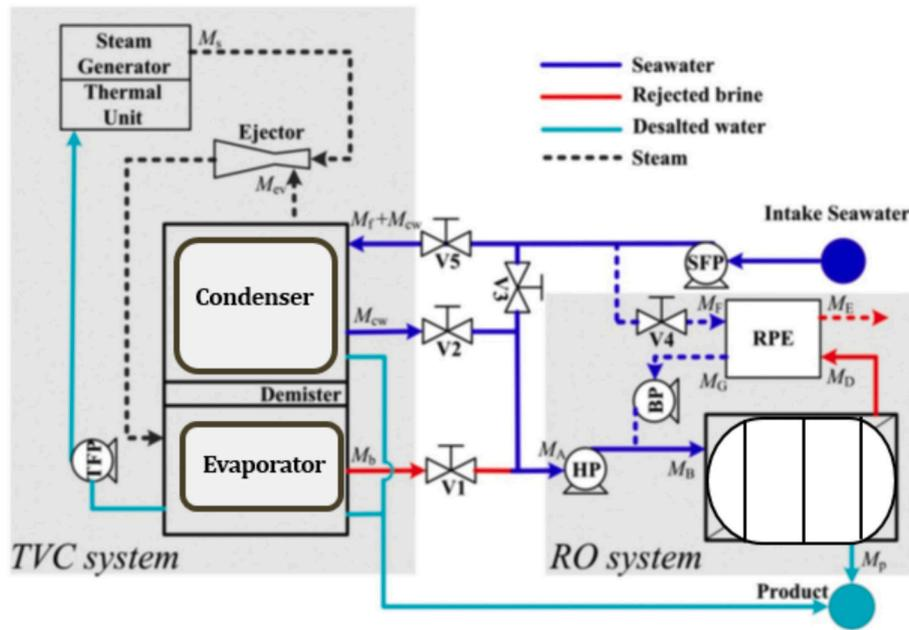
Fig. 22. A representation of an RO-TVC hybrid system with a pressure exchanger (Adapted from [53]).
