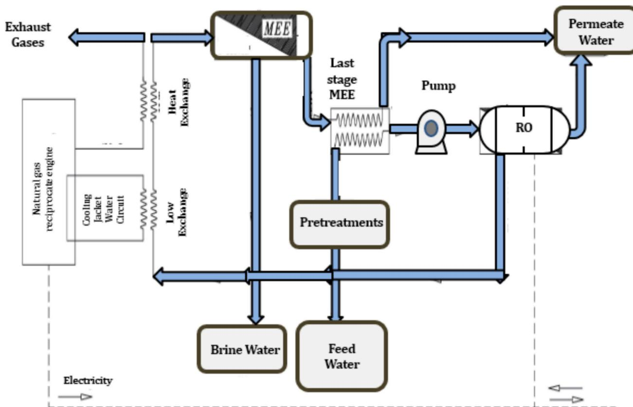
Fig. 17. A representation of the RO-MED hybrid system and NGRE to supply electricity and water (Adapted from [49]).
