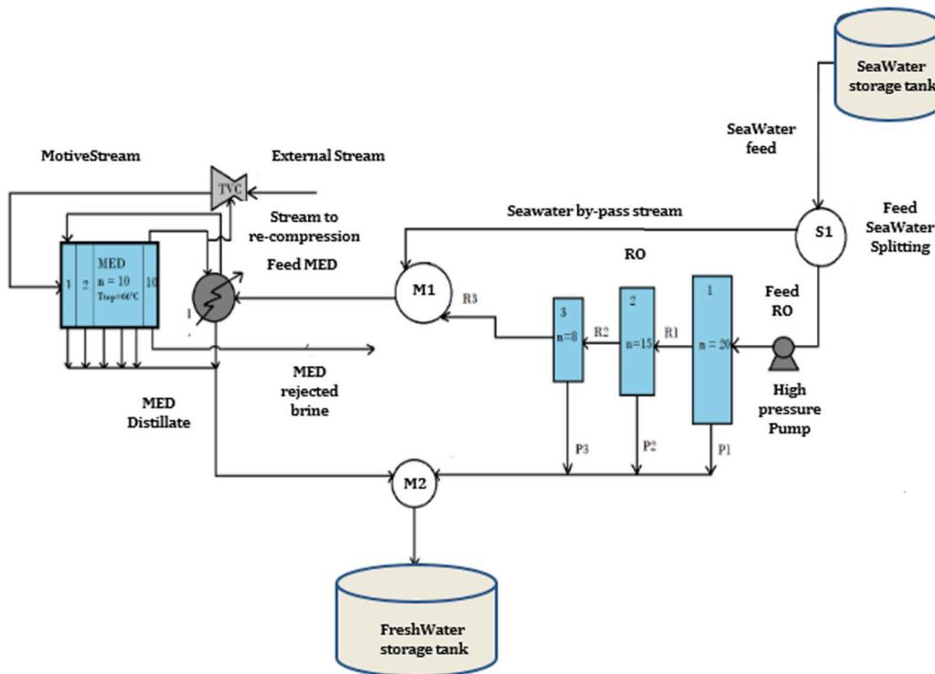
Fig. 21. RO upstream in the integrated RO-MED/TVC system (Adapted from [47]).
