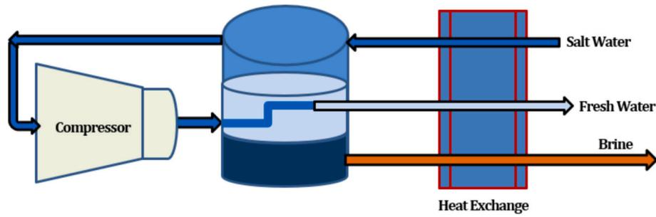
Fig. 5. A representation of thermal vapour compression (Adapted from [34]).
