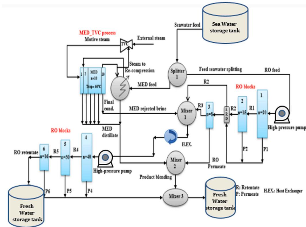
Fig. 31. A representation of integrated system of MED/TVC and double RO units (Adapted from [35]).
