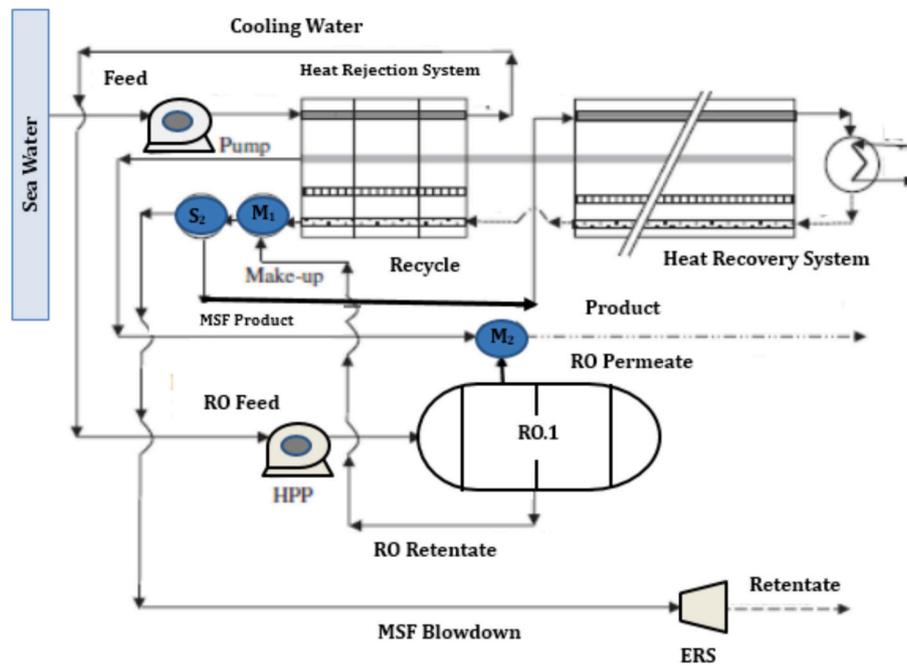
Fig. 15. A representation of one of the studied scenarios of the hybrid brine recycling MSF and a single-stage RO unit (scenario 5) (Adapted from [46]).
