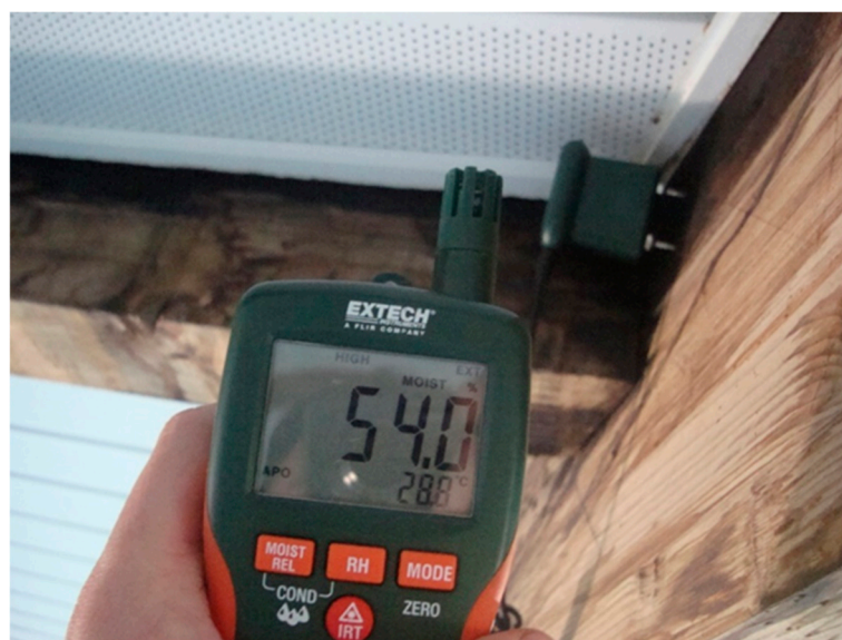
Figure 4. Measurement of wood temperature and moisture content with a needle thermohygrometer.
