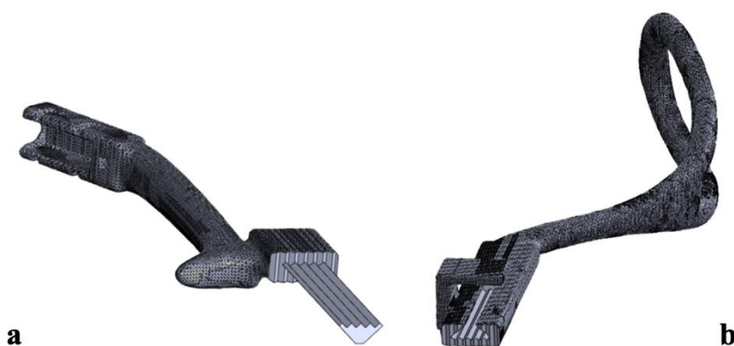
Figure 1: Forceps partition design using a) tang in handle and b) hollow in cephalic spoon.
