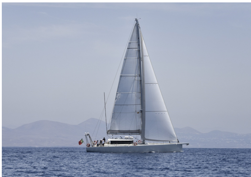
Figure 1. The S/Y Eugen Seibold under sails off Lanzarote Island. Air is sampled from ca. 13 m above sea surface at the top of the black tube behind the beam. Devices for sampling of the water column are deployed from the A-frame at the stern (see also Figure 3). Photo, D. Jack, MPIC.
