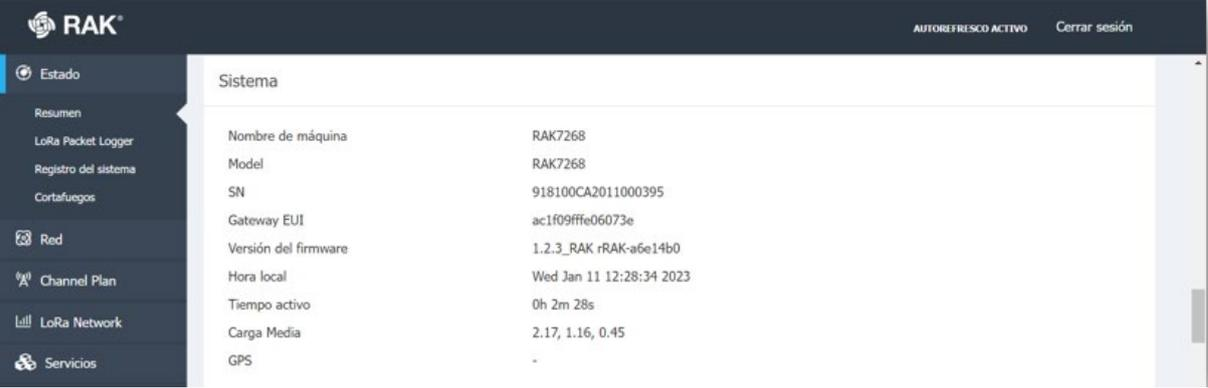
The screenshot shows the RAK web interface. The top navigation bar includes the RAK logo, 'AUTOREFresco ACTIVO', and 'Cerrar sesión'. A left sidebar contains menu items: 'Estado', 'Resumen', 'LoRa Packet Logger', 'Registro del sistema', 'Cortafuegos', 'Red', 'Channel Plan', 'LoRa Network', and 'Servicios'. The main content area is titled 'Sistema' and displays the following system information:
