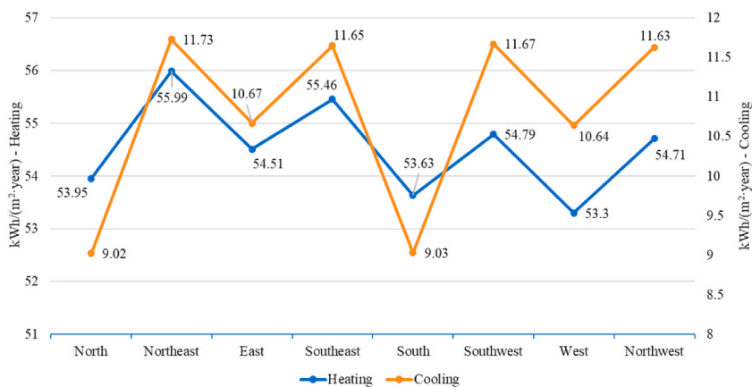
Fig. 3. Energy consumption of a single-family dwelling according to the orientation of its front façade. The example shown is the case of dwelling type H3, climate zone B2, façade type F3 and roof type R1.
