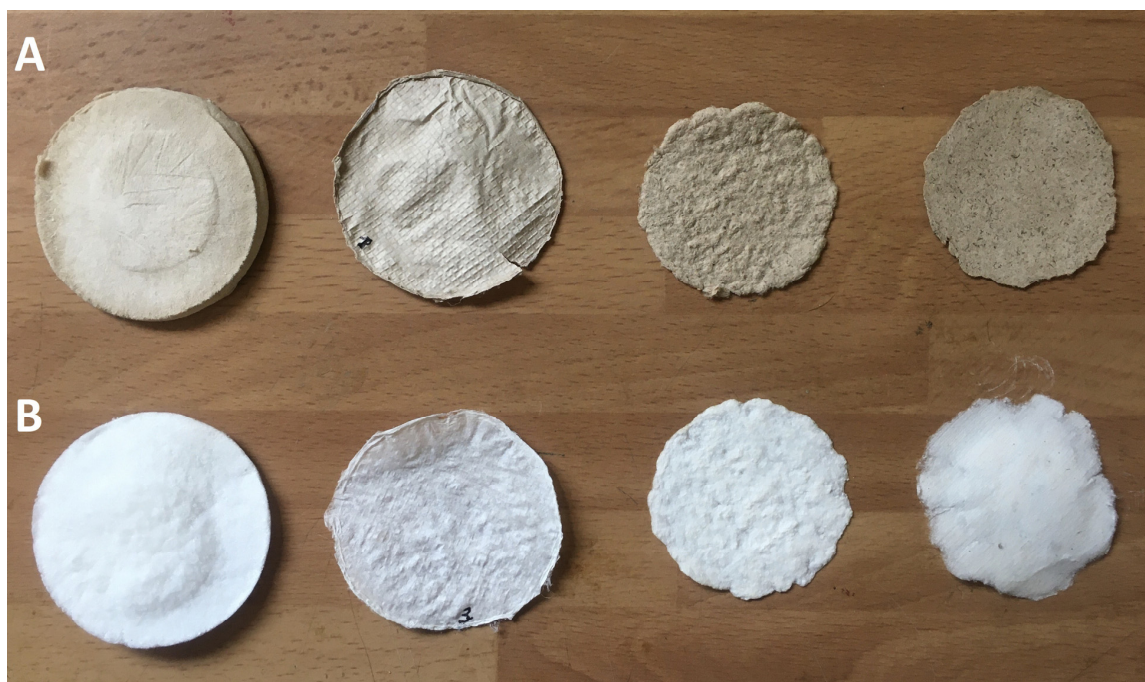
Figure 1. Filters obtained by each manufacturing process: freeze-dried, vacuum filtered, crushed, and pressed (from left to right). (A) row: alkali-treated pulp. (B) row: from bleached pulp.
