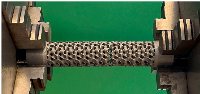
Fig. 10. Photograph of the torsional test of one of the scaffolds.
